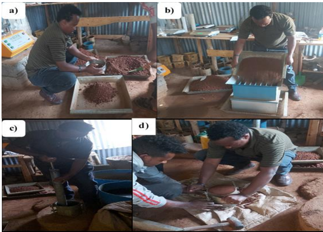
Figure 3-7: standard compaction test (a) sample preparation (b) sample quartering (c) compacting (d) compacted sample trimming
