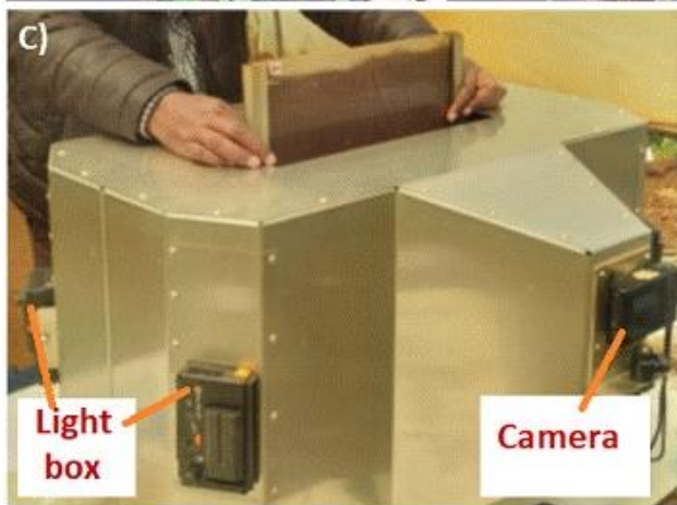
Appendix 8.3. The experimental procedure. A) Root chambers covered with polycarbonate sheet to protect the roots from light; B) A microscope for measuring stomata related traits and counting the number of root hairs; C) Imaging box with mounted camera and light box; D) Measuring nodal root angle
