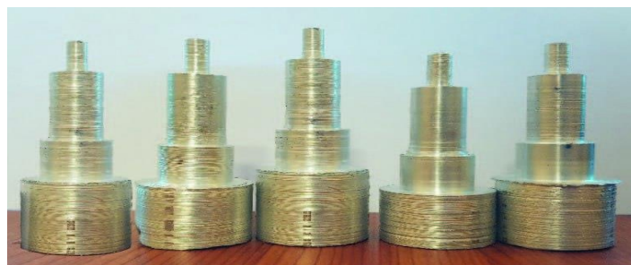
Figure 3-17 Fabricated Al7075-based hybrid composite samples (S1–S5) after turning operation.
