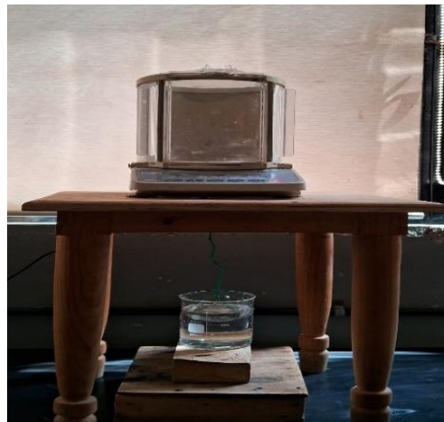
Figure 3-18 Measurement of experimental density in distilled water
