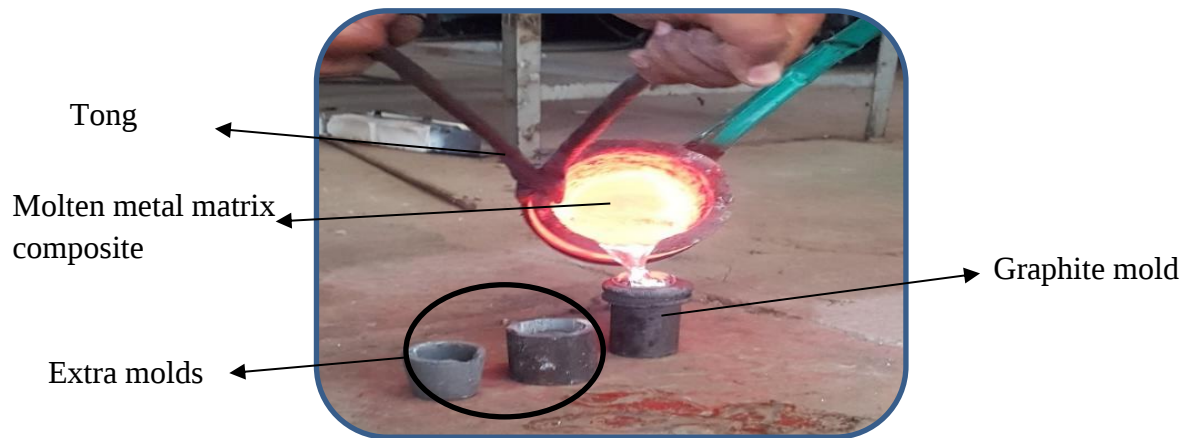
Figure 3-14 Poring of the melt composite in to the mold
