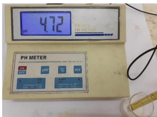
Figure 3. 1: pH determination of Euphorbia trigona Mill latex with a digital pH meter
