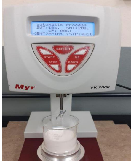
Figure 3. 3: Determination of Viscosity of Euphorbia Trigona Mill latex with digital viscometer
