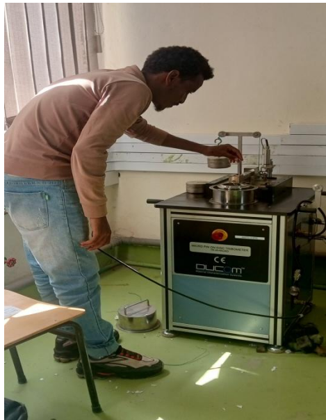
a) Wear testing
