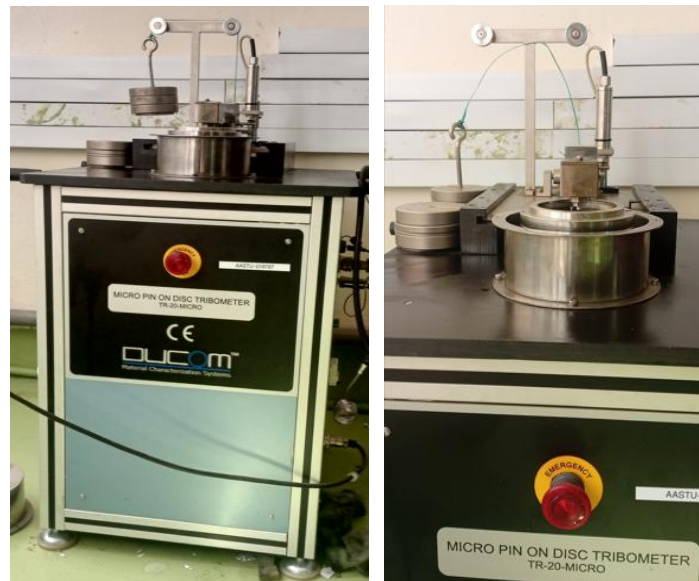
Figure 3.12 Micro pin on disc tribometer used for wear testing (located in AASTU)
