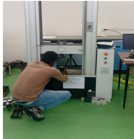
a) Compression testing (sample dimension was prepared as per ASTM E9, d=12.7\text{mm} , h=18\text{mm} )
