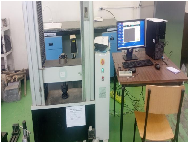
a) Compression testing (sample dimension was prepared as per ASTM E9, d=12.7\text{mm} , h=18\text{mm} )
