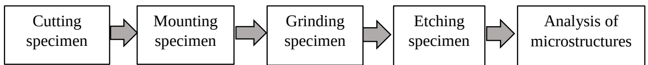
Figure 3.13 Procedure of specimen preparation metallographic test
