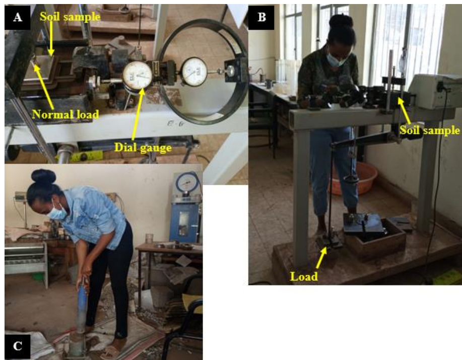
Figure 3. 5 Figure showing a direct shear test of soil in the laboratory.
