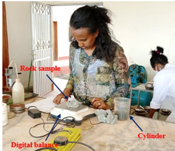
Figure 3. 3 Unit weight test on an irregular rock sample.
