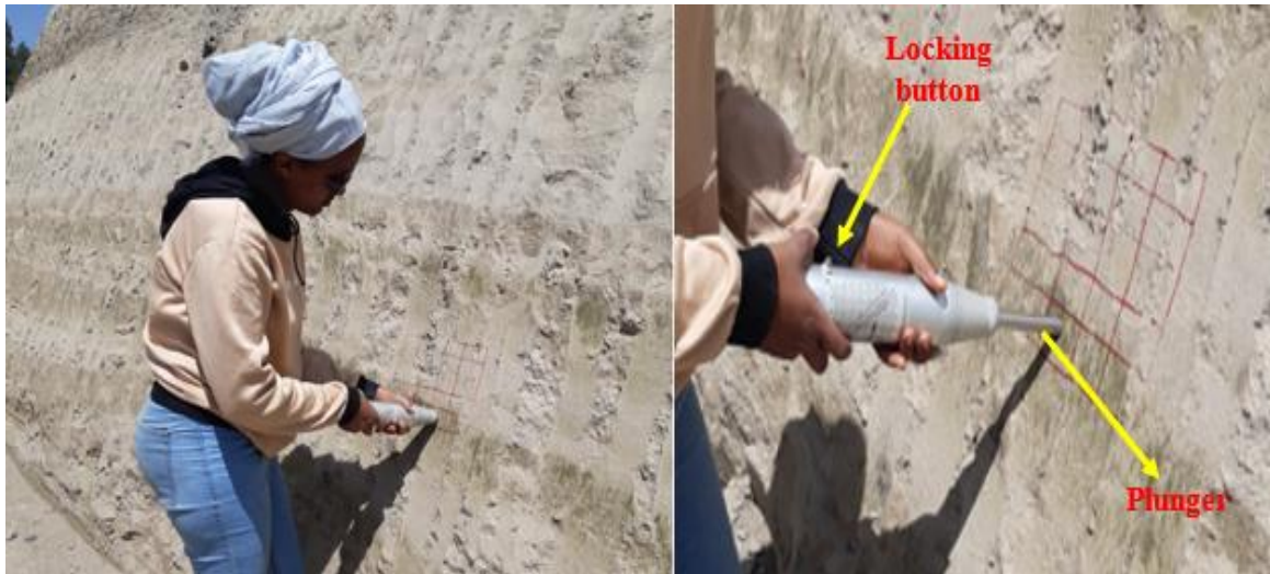
Figure 3. 2 Insitu strength test.
