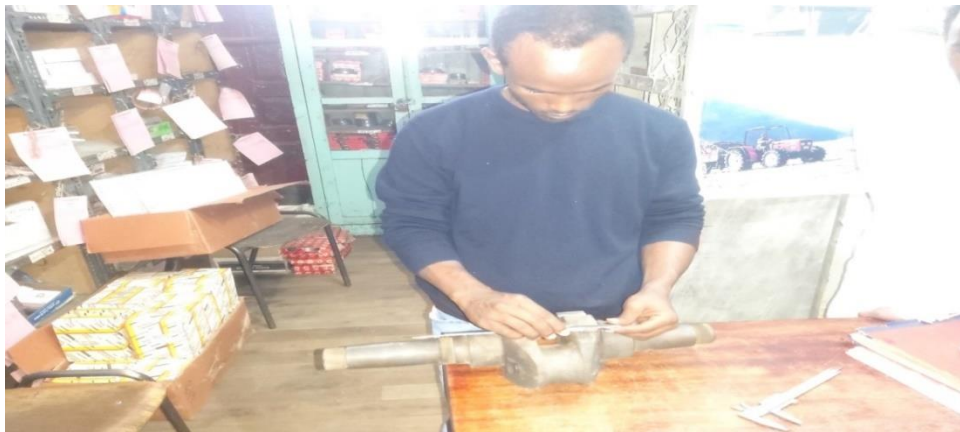
Figure 3.2 Photo of measuring crank shaft of JSD 1800
