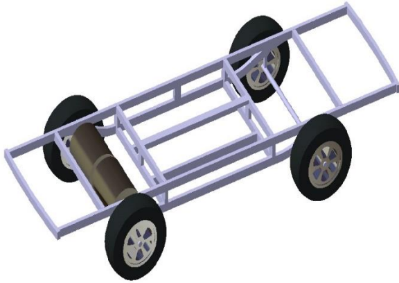
Figure 4-6 Designed electric vehicle chassis frame (ladder type)
