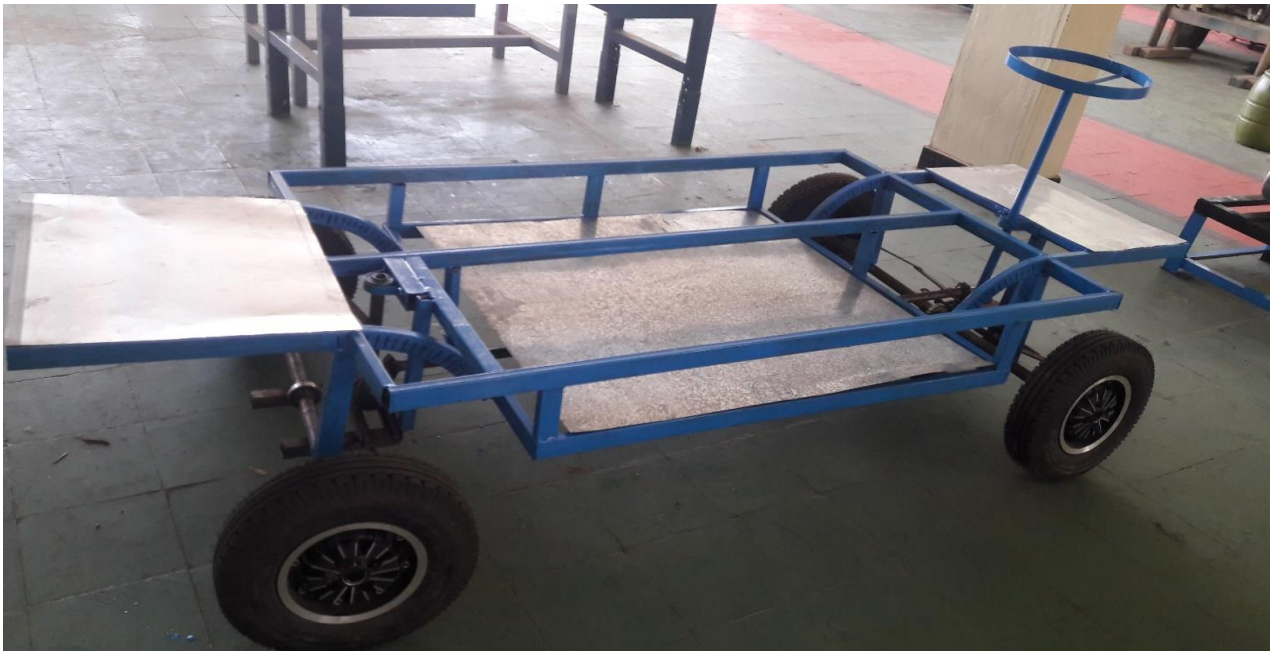
Figure 3-3 Chassis frame for designed electric vehicle
