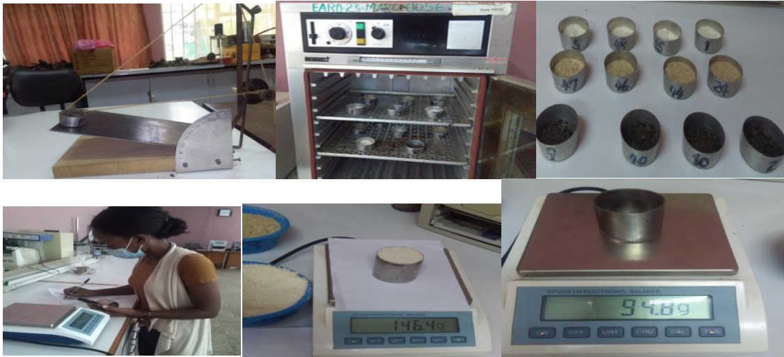
Measuring angle of repose, moisture contents and bulk density of feed samples.
