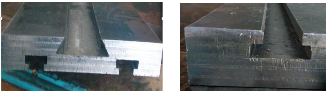
Figure 3-8 Grooves in column support
