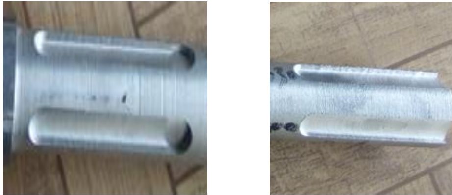
Figure 4-6 Keyway end milling of Aluminum shaft by fixture and vertical milling fixture
