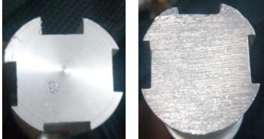
Figure 5-7 Keyway milling on shaft a) by milling machines b) by fixture
