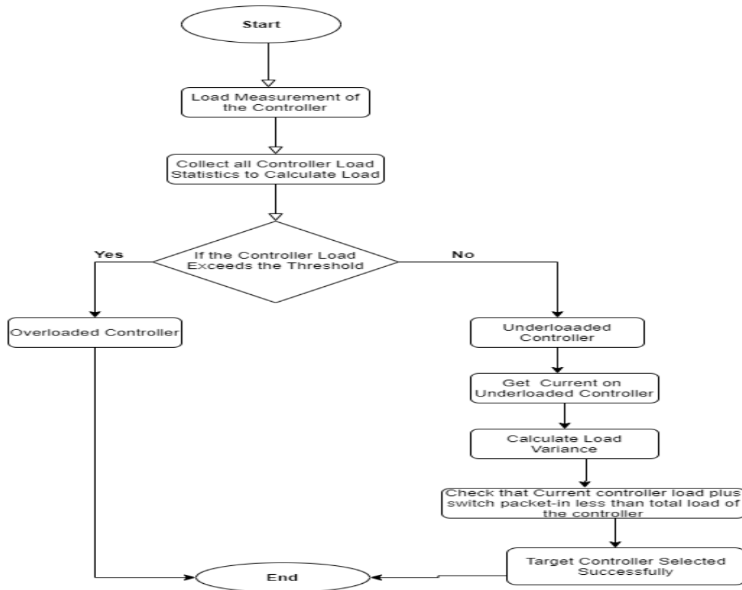
Figure 3.5 Flowchart of Controller Selection
