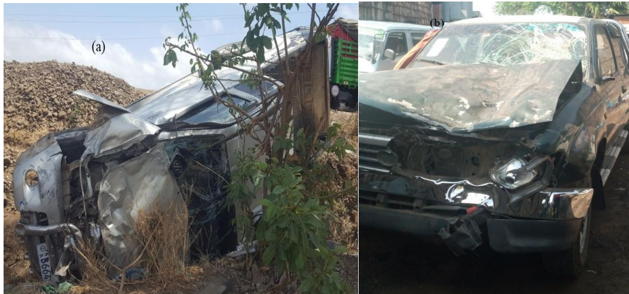
Figure1.1: (a) side collision which causes rollover (b) Front collision of pickup vehicle
