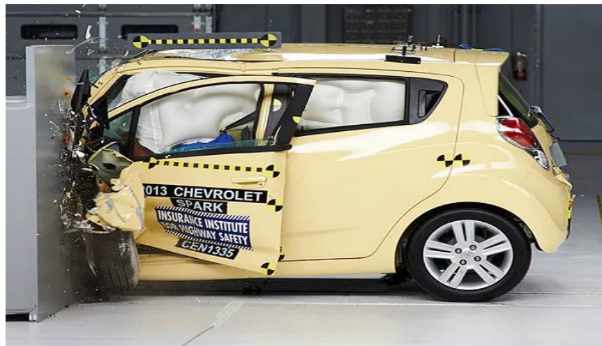
Figure 2.6: The IIHS tests a Chevrolet Spark ("NHTSA Crash Test - Consumer Reports," 2014)
