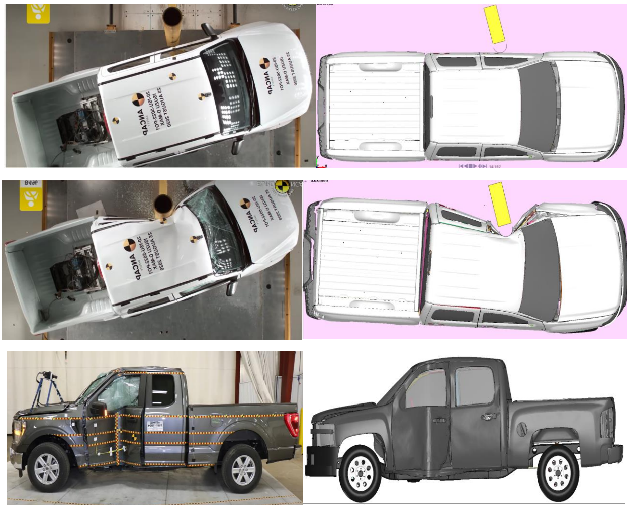
Figure 5.54: Sequence of side pole crash FEA Vs real NCAP crash test
