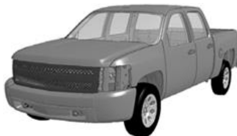
Figure 2.14: FE model of pickup (Park et al., 2013)
