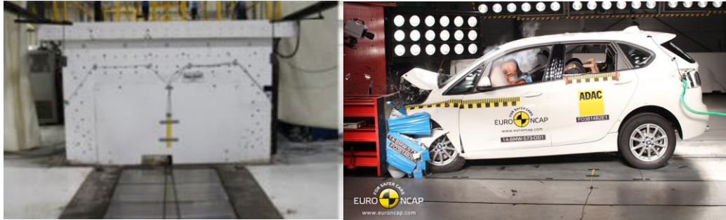
Figure 2.7: Test set up and the post-crash vehicle of the NCAP frontal crash (Singh, 2012)
