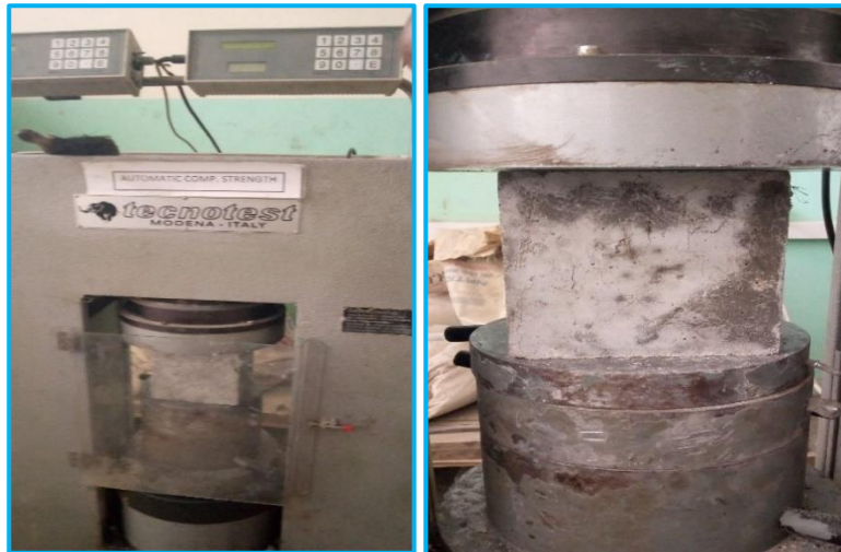
Figure 3.9 Compressive strength test setup
