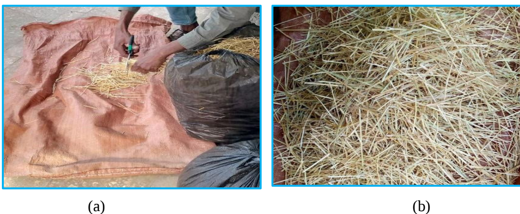
Figure 3.1 a) Cutting teff straw using a pair of scissors, b) Teff straw washed and air-dried
