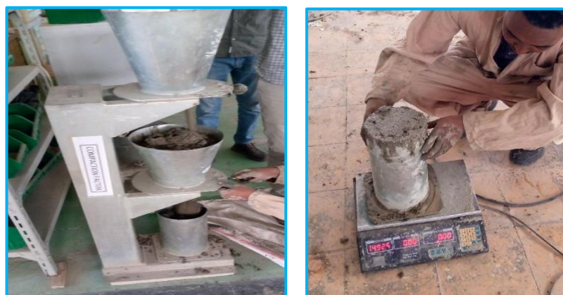
Figure 3.7 Compaction factor test
