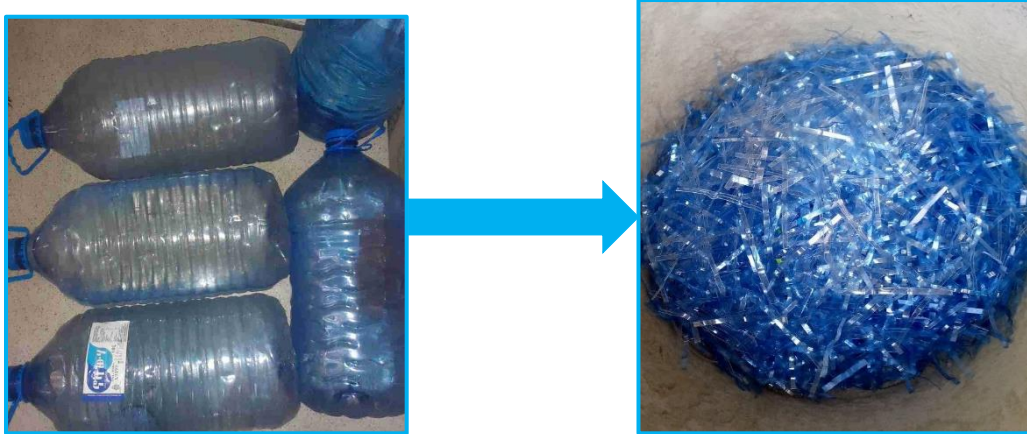
Figure 3.2 Preparation of PET fibers
