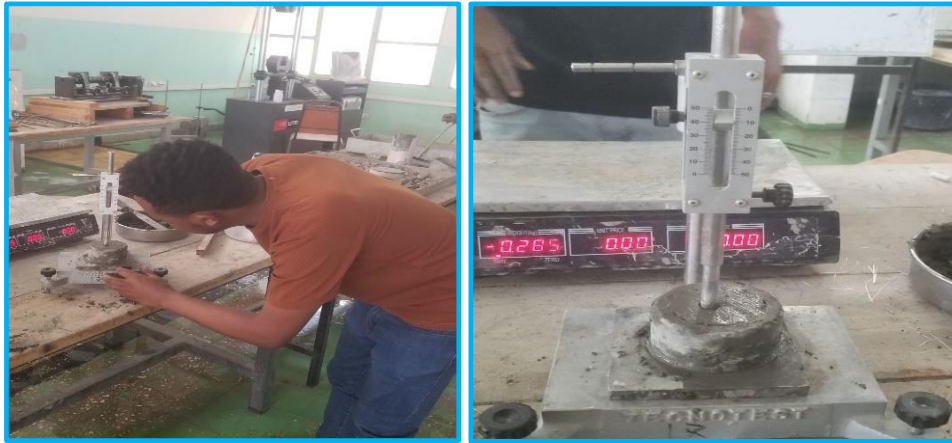
Figure 3.4 Normal consistency of cement test
