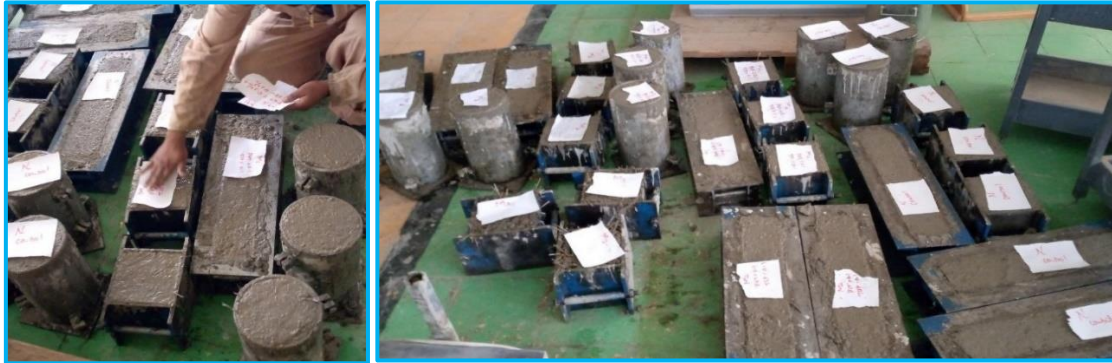
Figure 3.8 Concrete Casting and marking
