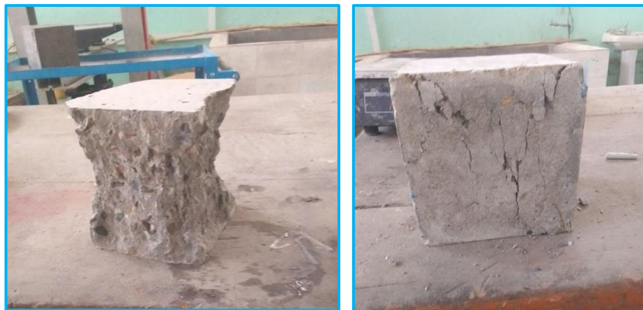
Figure 4.7 Test specimens which failed under compression, (a) control, (b) HFRC
