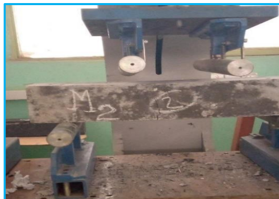
Figure 3.10 Flexural strength test setup
