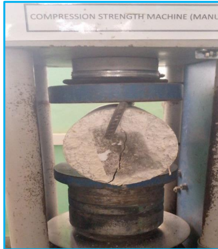
Figure 3.11 Splitting tensile strength test setup
