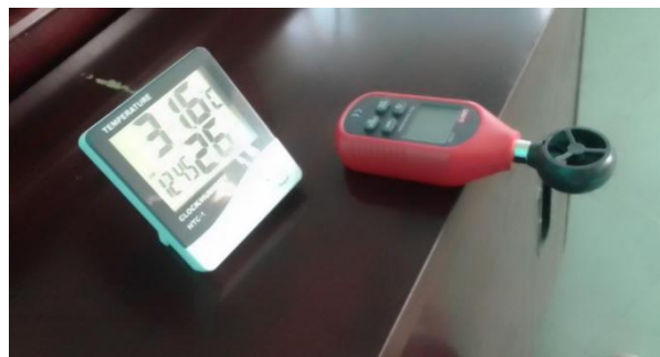
Figure 3.20: Digital data logger and Anemometer
