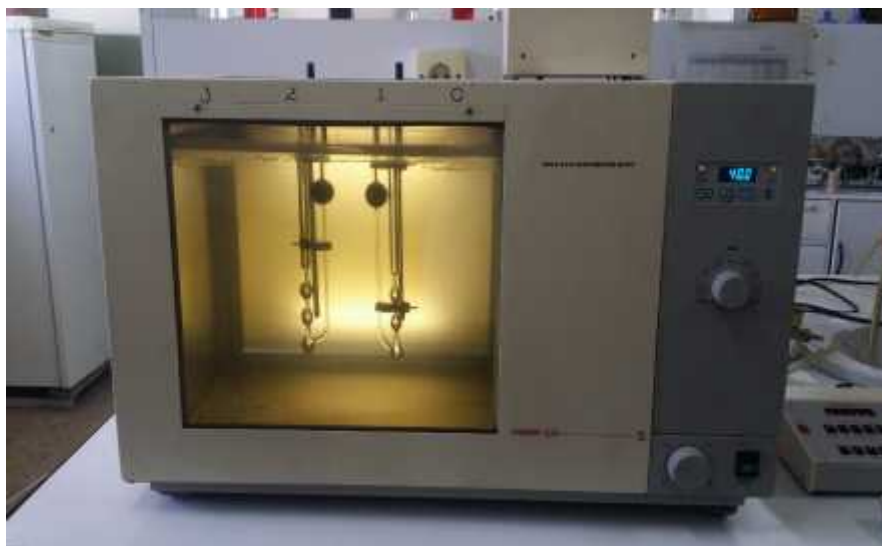
Figure 24: Cannon-Fenske style glass capillary tube in a SETA.KV-8 viscometer bath.
