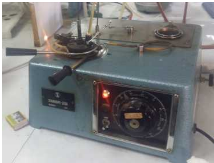
Figure 25: Test cup and Pensky-Martens Closed Cup Flash Point Testing Machine
