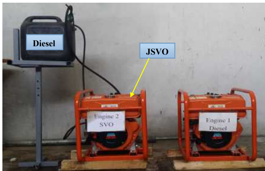
Figure 21: Overall picture of experimental setup for dual fueling and diesel engine
