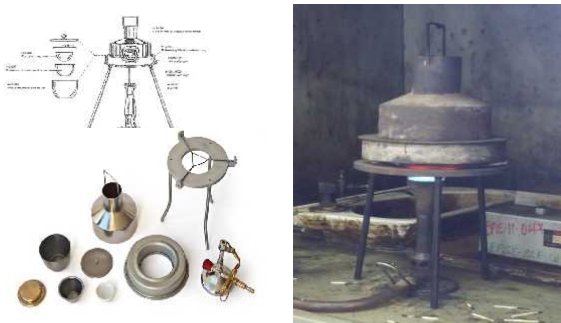
Figure 29: Conradson Carbon Residues Apparatus and Carbon Residue Tester (Conradson Method)
