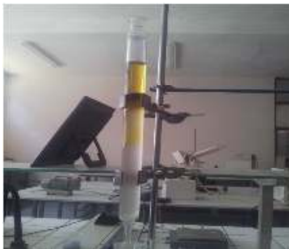
Fig 8: Column chromatography analyses of chloroform crude extract with chloroform/methanol solvent system
