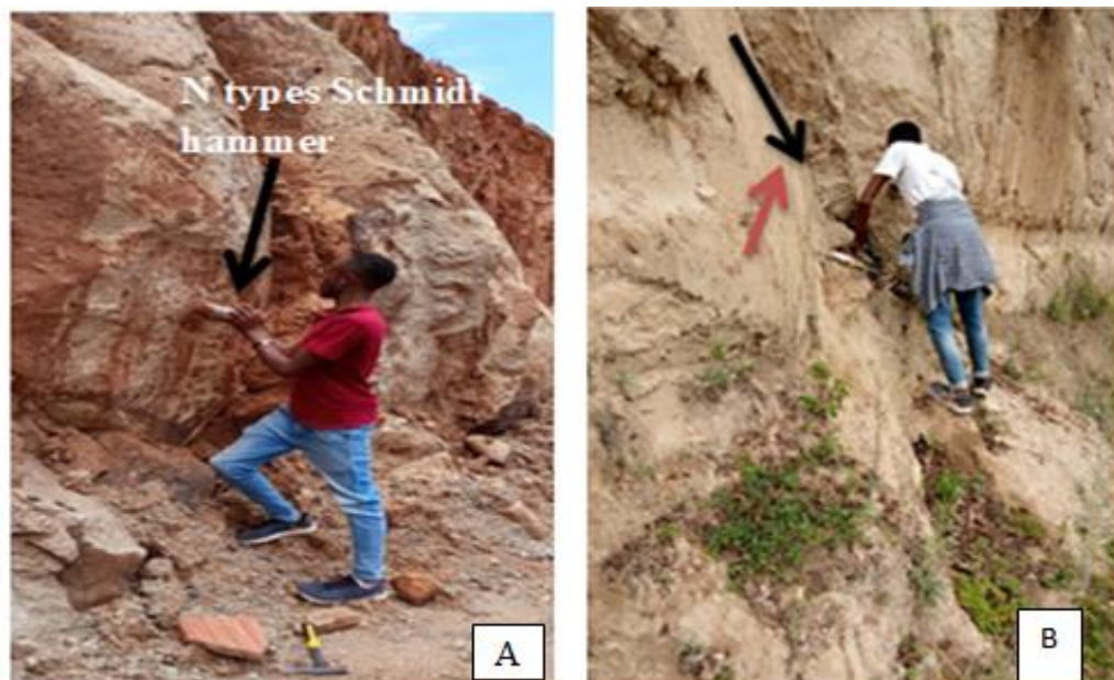
Figure 17: Conducting Schmidt hammer on ignimbrite rock in the study area (A) at GPS reading (long. 430552m lati.745141 m). (B) Measuring orientation of dip for joints by using a compass at GPS reading (long. 437833 m lati.745374 m).
