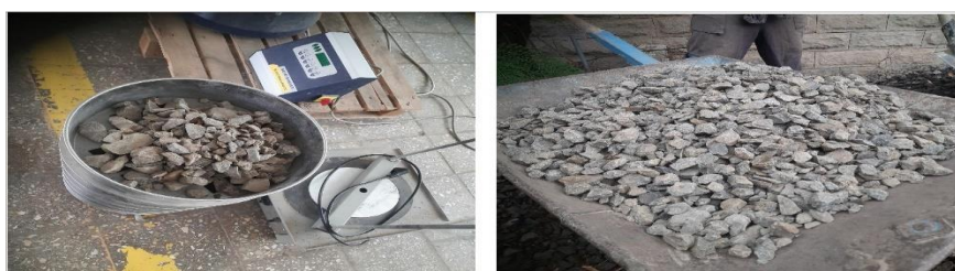
Gradation of coarse aggregate
