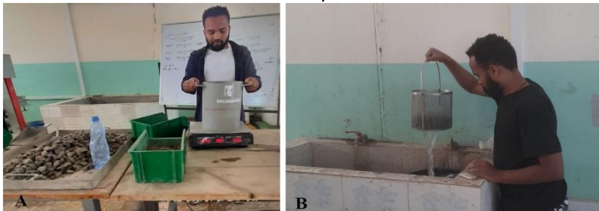
A) unit weight of coarse aggregate, B) specific gravity of coarse aggregate
