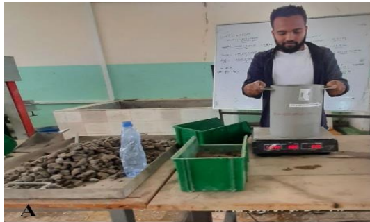
A) unit weight of coarse aggregate, B) specific gravity of coarse aggregate
