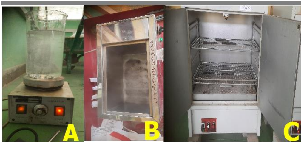
Figure 4.25 A) string NaOH and Zinc, B) Bathtub washing, C) open-air oven dry
