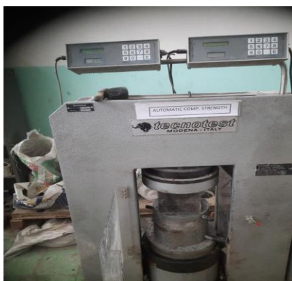
Automatic Compressive Test Machine (a), Compressive Strength Test (b)
