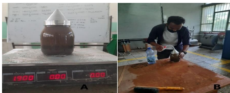
Scoria sample(A) and sand sample(B) on determination of specific gravity
