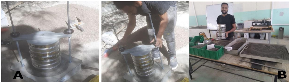
Gradation test for Fine aggregates sand(A) and scoria(B)
