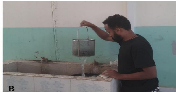
A) unit weight of coarse aggregate, B) specific gravity of coarse aggregate
