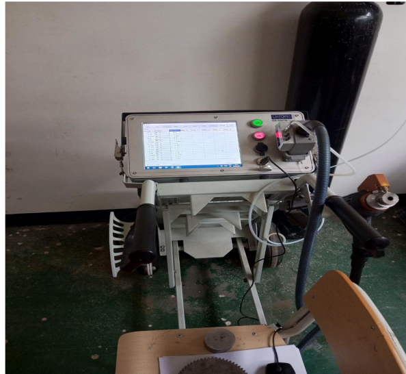
Figure 3-3 spectroscopy used to identify chemical composition
