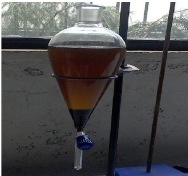
Figure 3.4. Glycerin settled at the bottom
