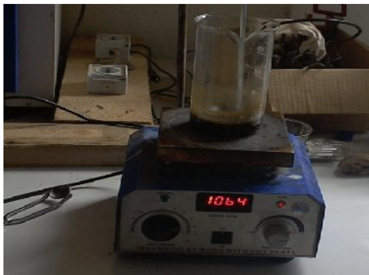
Figure 3.3. Heating of crude oil
