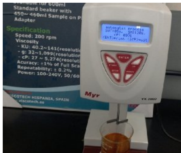
Figure 11. The viscometer set up
