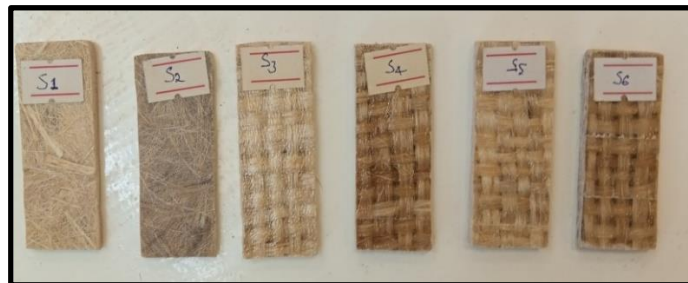
Figure 3.19 Hardness test samples.
