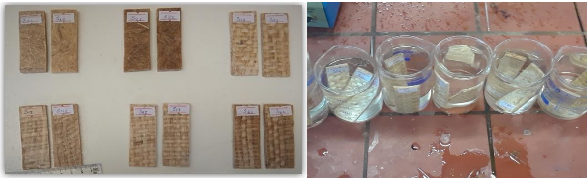
Figure 3.21 Specimens for water absorption test and under test.
