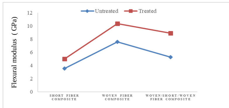
Figure 4.12 the effect of alkaline treatment of flexural modulus of banana fiber polyester composite.
