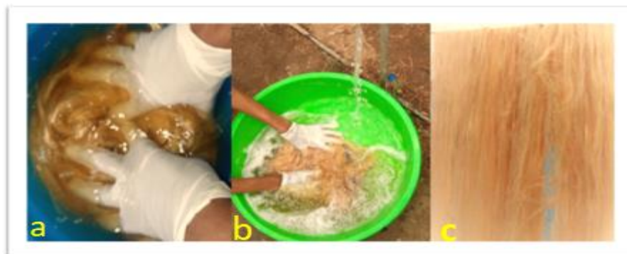
Figure 3.4 a) NaOH treatment b) washing fiber c) Drying under sunlight.
