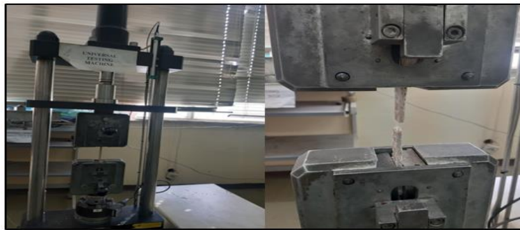
Figure 3.13 Specimen under tensile test.
