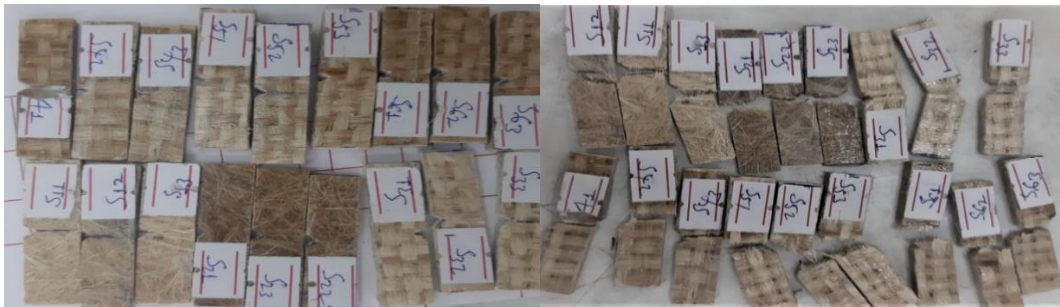
Figure 3 18 Specimens before and after impact test.
