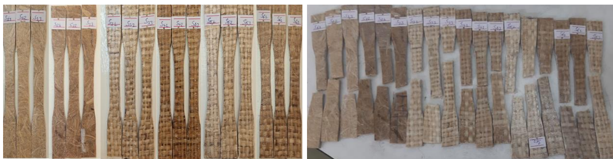
Figure 3.14 Tensile test Specimens before and after test.
