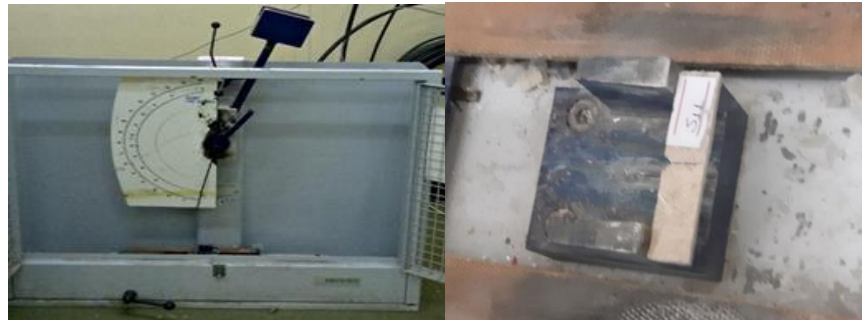
Figure 3.17 Specimen under impact test.
