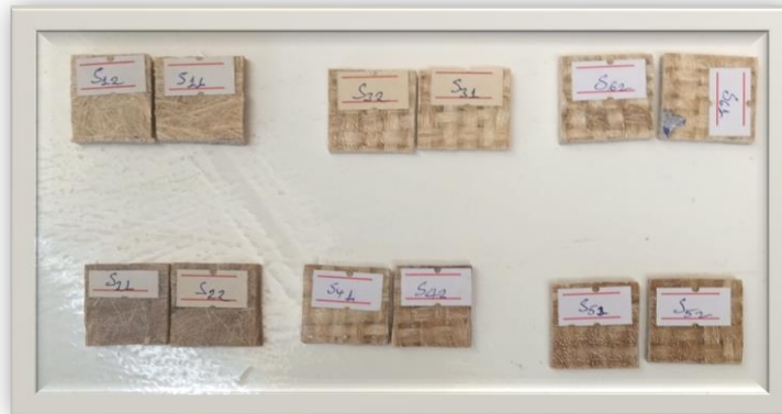
Figure 3.20 Specimens for void content determination.
