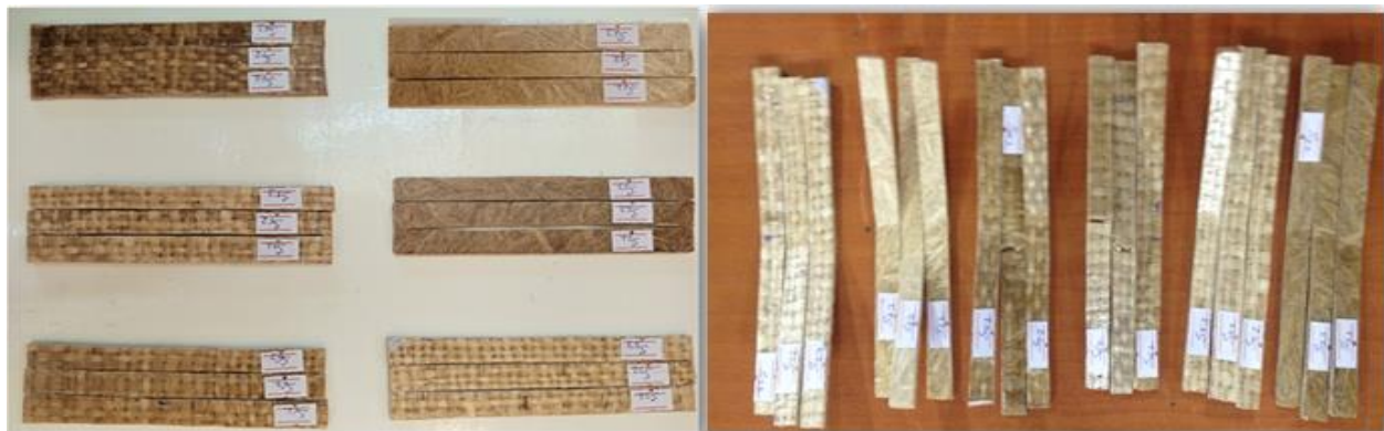
Figure 3.16 Flexural test specimens before and after test.
