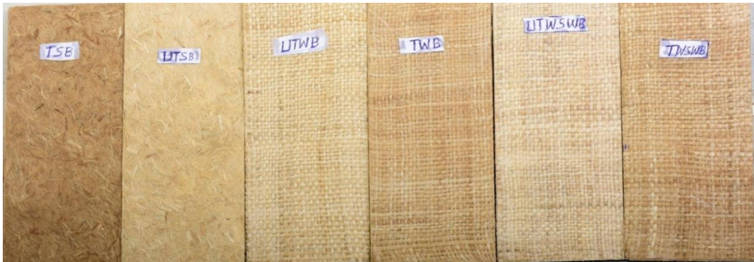
Figure 3.12 Banana fiber polyester composite samples.
