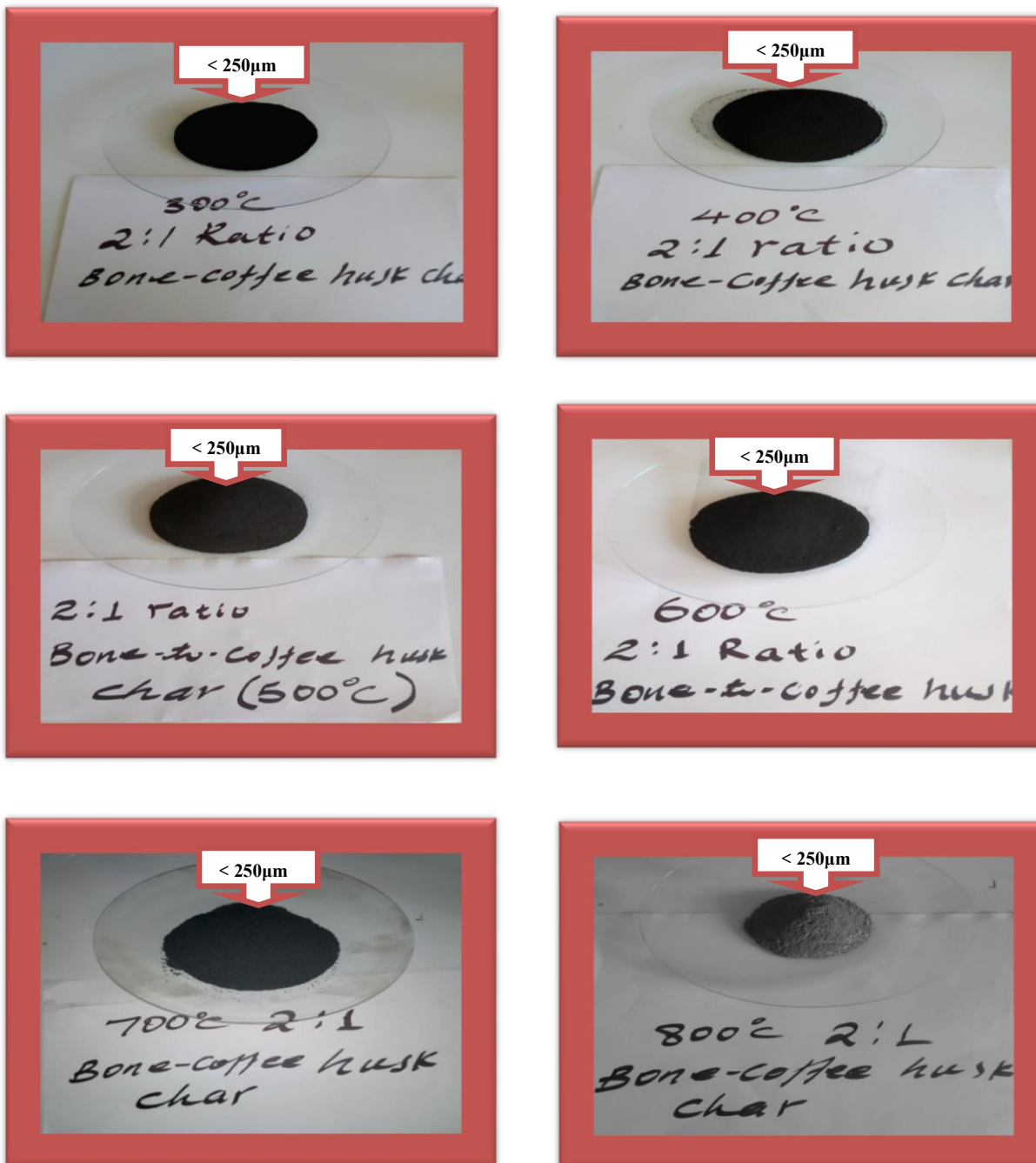
Figure 4.1 Charcoal obtained from bone and coffee husk at different pyrolysis temperature
