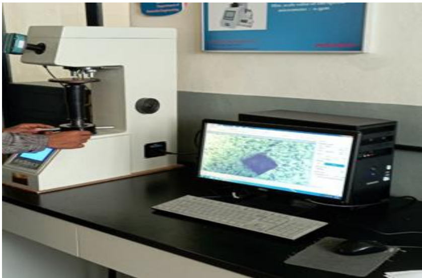
Figure 3-16 Vickers hardness testing machine set up
