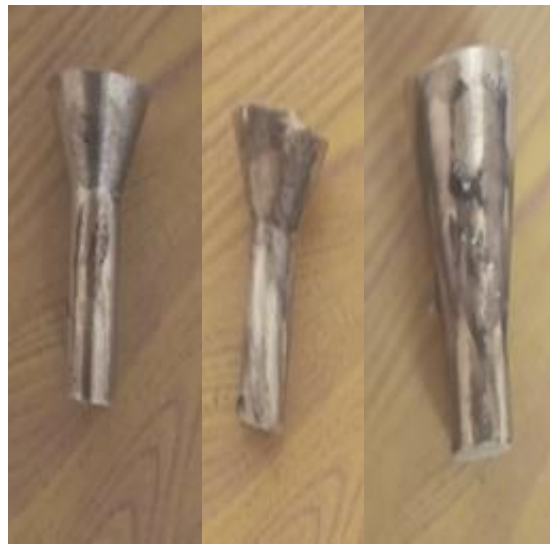
Figure 3-14 Extruded samples of cosine, linear convergent and streamline respectively
