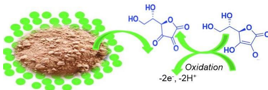
Figure 66. The proposed mechanism of electrochemical oxidation reactions for electrocatalytic oxidation of AA to dehydro-ascorbic acid at the NCs sensor (Murugan et al., 2019).
