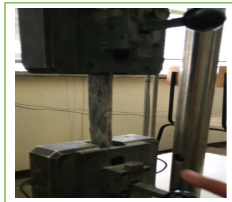
Figure. 3.14. Typical tensile specimen under tensile test.
