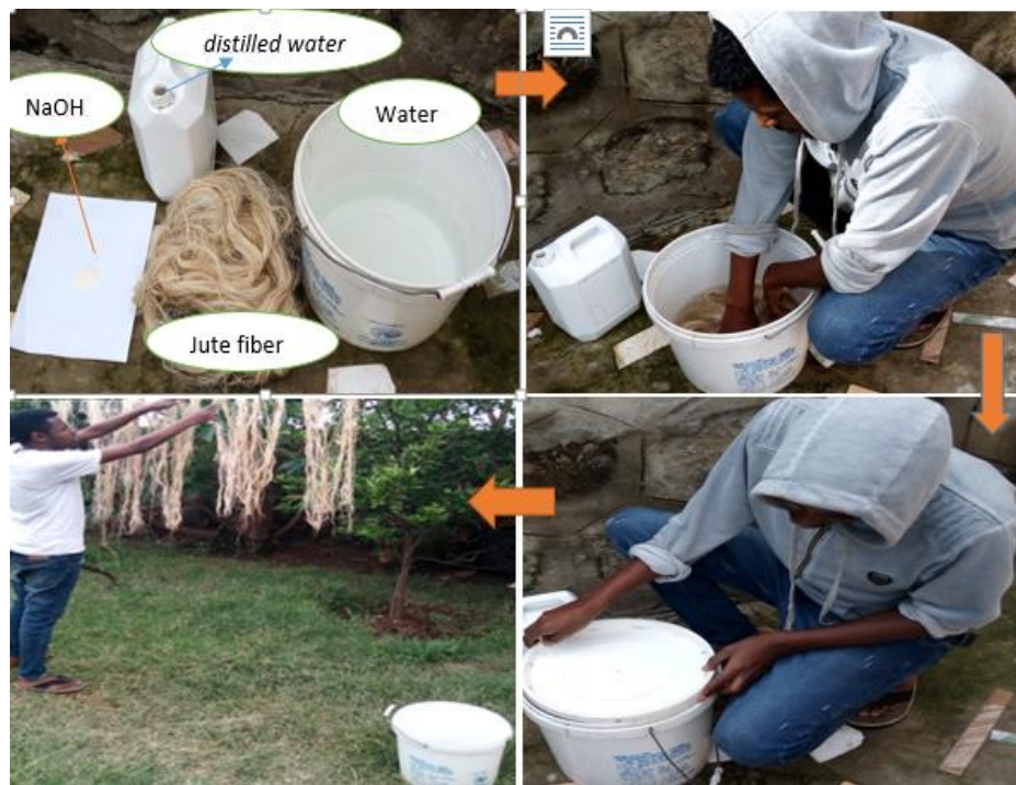
Figure. 3.4. Alkaline treatment of jute fiber.
