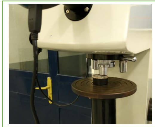
Figure. 3.16: Micro- hardness measurement under Vickers Hardness Tester (HVS-50)
