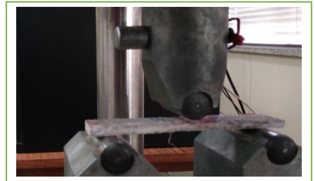
Figure. 3.15. Three-point bending 1- load probe, 2- support, 3- specimen, d- depth of specimen, L- support distance (span) and S- overall length of specimen
