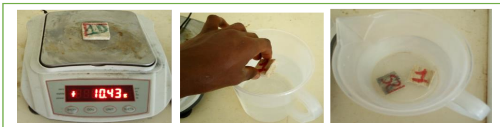
Figure. 3.13. Al_2O_3/SiC filled JFRPC sample in the rain water for one day.
