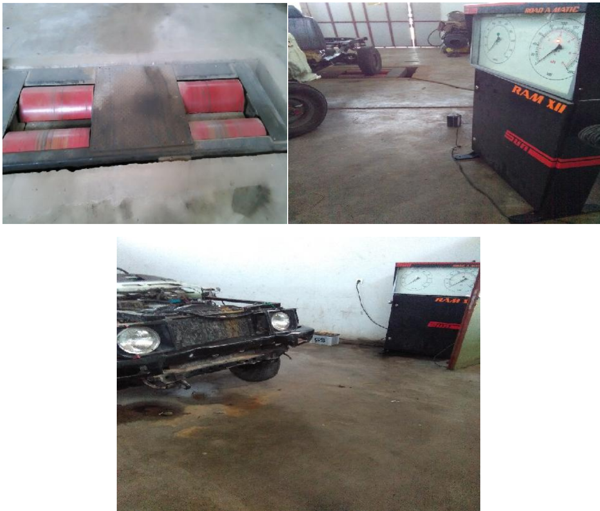
Figure 3.26. Chassis dynamometer and vehicle for performance test
