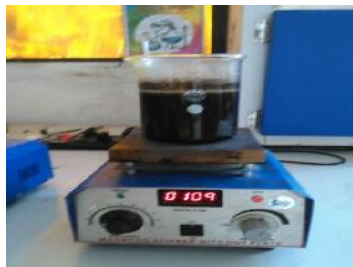
Figure3.4. Heating the mixture of (KOH & methanol) with crude oil.
