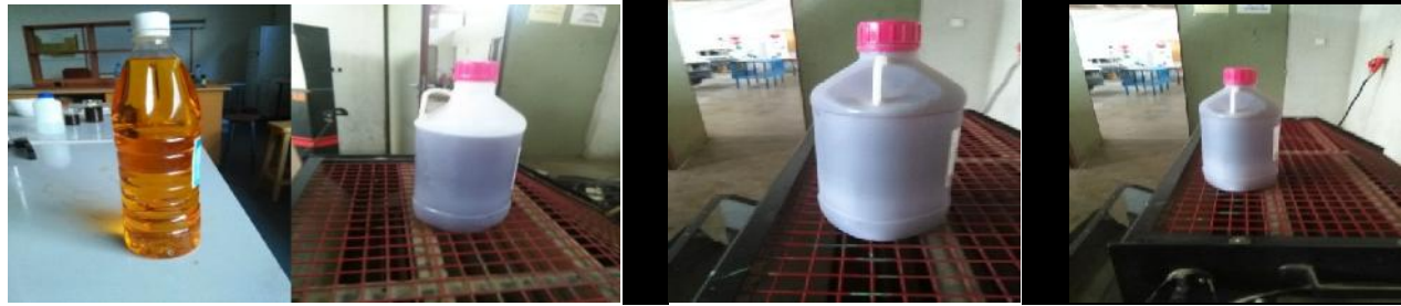
Figure3.23 From left to right B100, B10, B20, B30 blend of biodiesel ready for performance test
