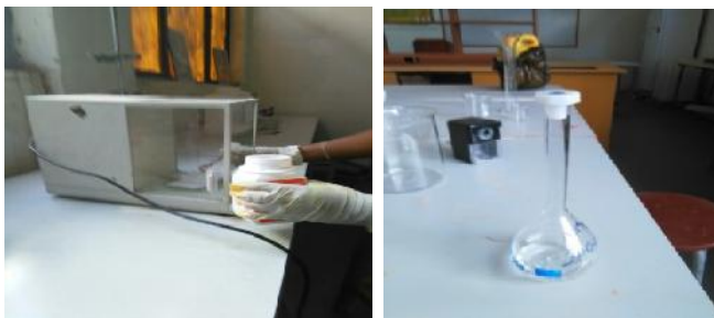
Figure3.2. Measuring KOH & dissolve it in methanol
