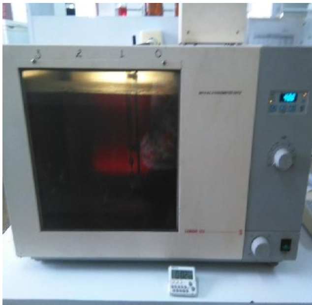
Figure.3.20. Kinematic viscosity apparatus & cannon fenske capillary viscometer tube
