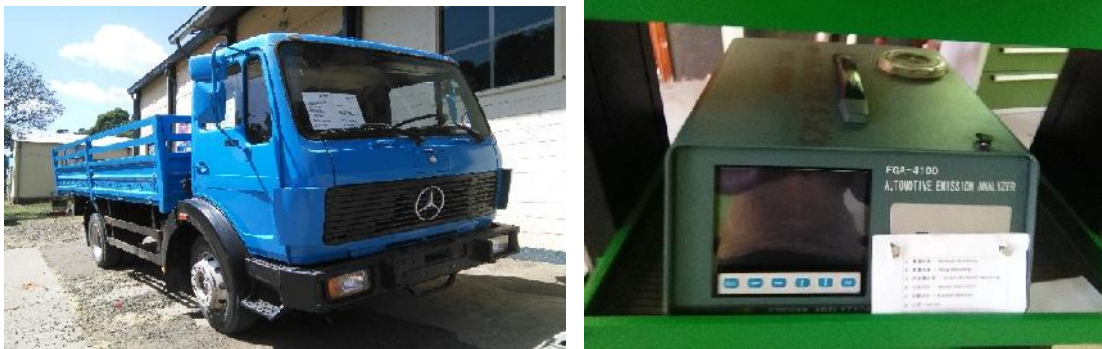
Figure 3.25. Vehicle & emission analyzer for exhaust gas measurement
