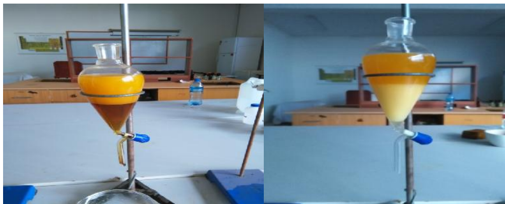
Figure 3.8. 1 st & 2 nd step of washing of biodiesel with distilled water (soap formation)
