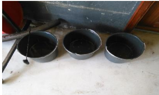
Figure 3.24. From left to right B10, B20, B30 blends of fuel for emission test
