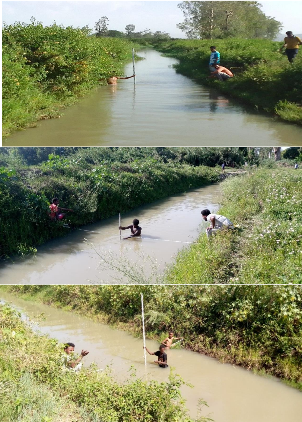
Figure 4.3 Right branch canal characteristics and discharge estimation
