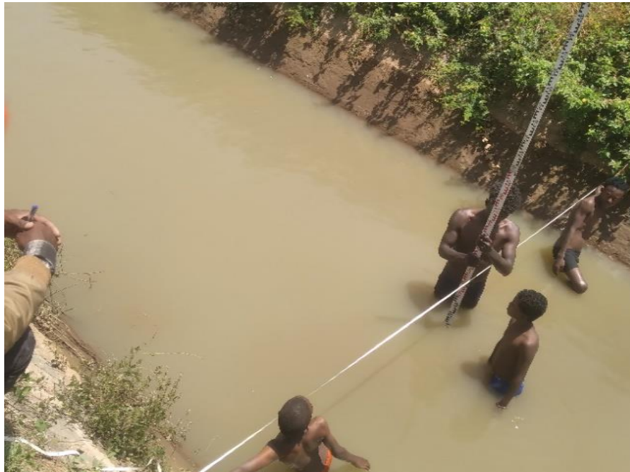
Figure 3.4 Main canal dimension and discharge measurement by float-area methods
