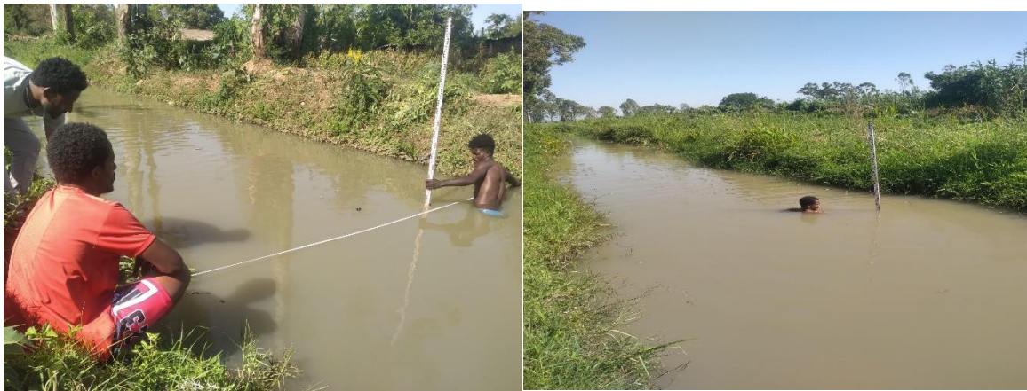
Figure 4.6 Water velocity measurement and canal dimension
