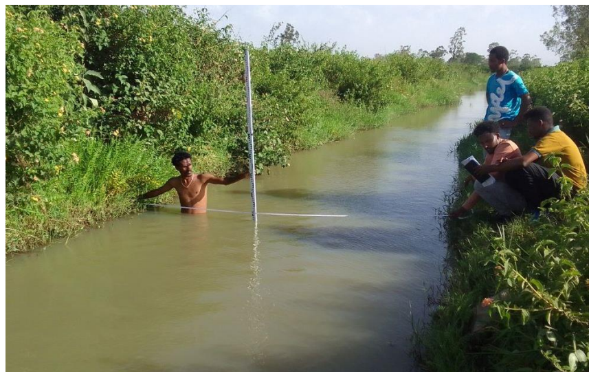
Figure 3.6 Discharge and secondary canal dimension measurement
