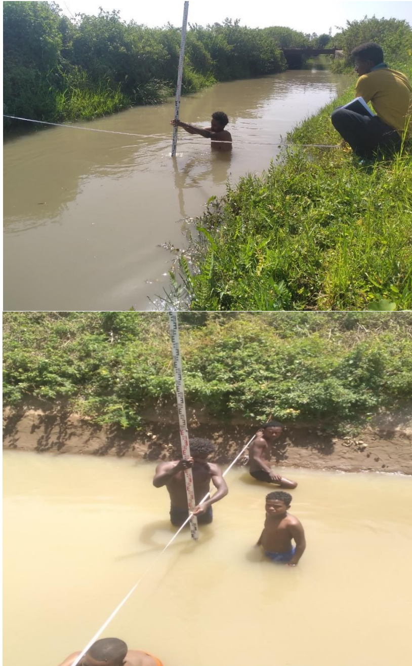
Figure 4.9 Main canal discharge measurement and canal dimension at water marked
