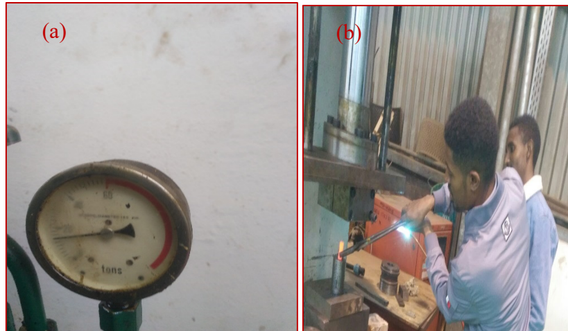
Figure 3. 13 The extrusion process performed on C15000 copper alloy using a 150-ton hydraulic press (a) Ton reading (b) Arranging in press machine
