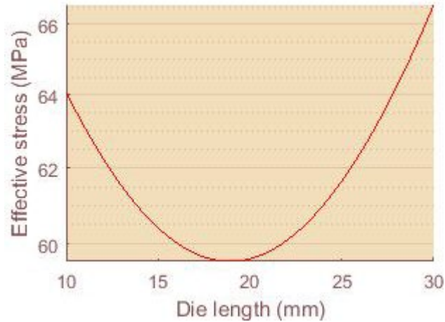
Figure 4. 15 Effective stress versus die length graph
