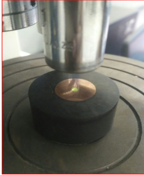
Figure 3. 18 Vickers hardness testing of C15000 material
