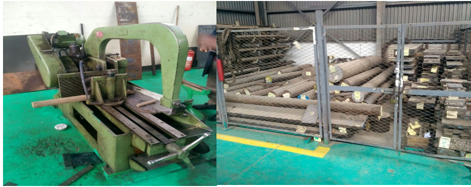
Figure 3. 11 Die material selection cut into the piece using a hacksaw
