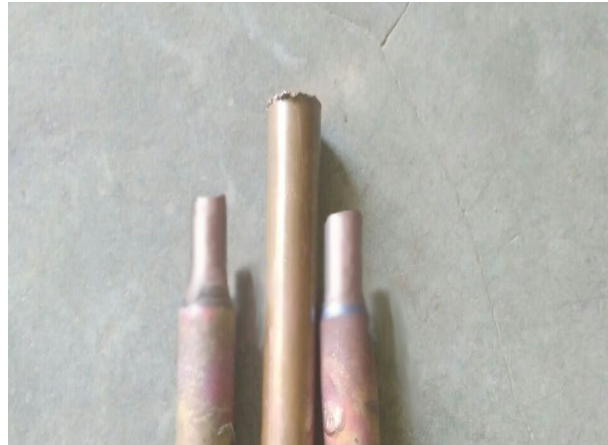
Figure 3. 15 Samples and extrusion components after the extrusion process
