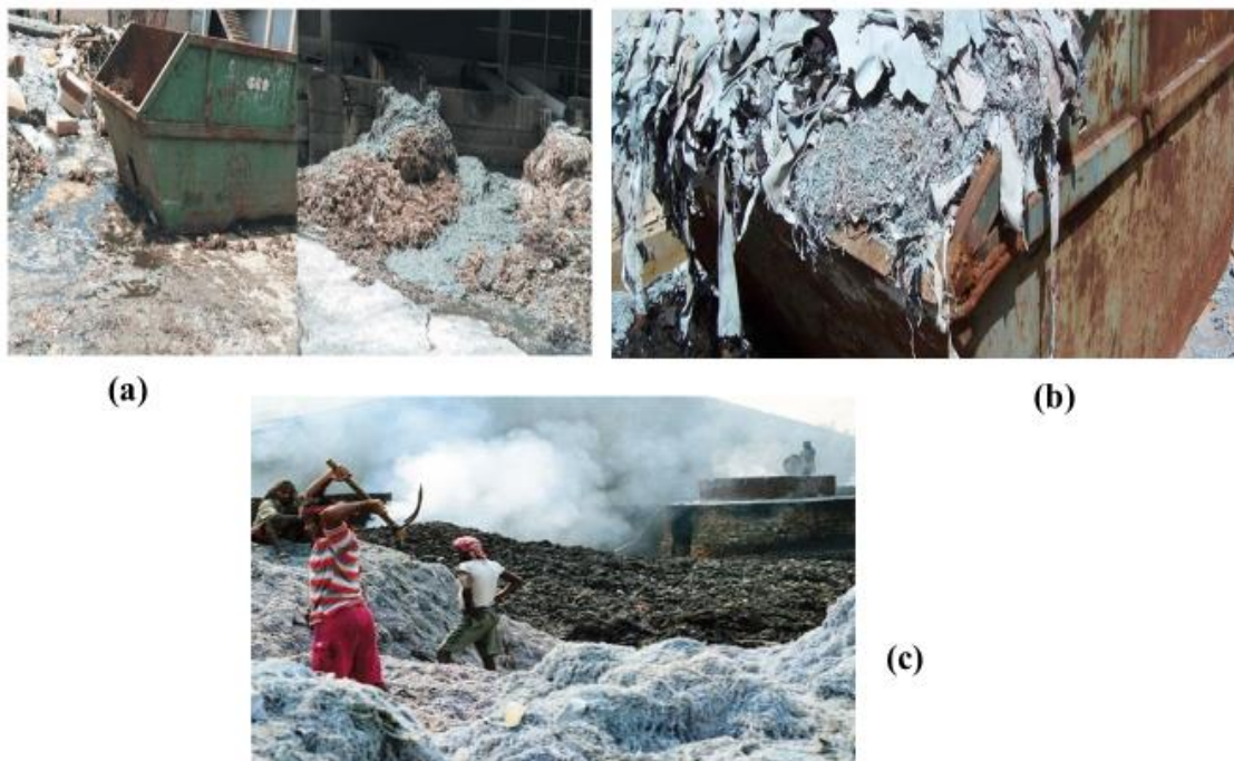
Figure 1: Solid waste management practices in the leather tanning industry: (a) accumulation of leather scraps in open bins, (b) close-up of chrome-tanned "wet blue" shavings, and (c) workers handling the open burning of solid waste without protective equipment (Basak et al., 2020).
