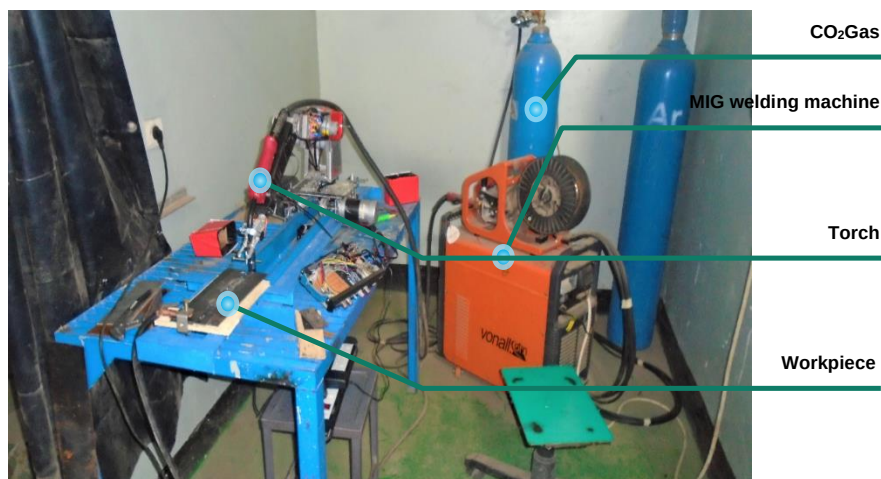
Fig 4.1 Overall arrangements of robotic arm with MIG welding machine
