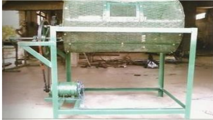
Figure 2.4. Pictorial view turmeric polishing machine (Moghe, 2012)
