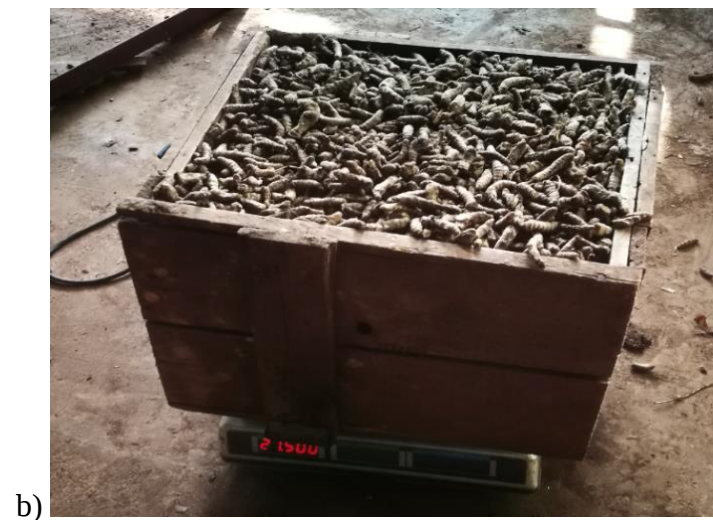
Figure 1. Turmeric rhizome a) width measurement b) Bulk density measurement
