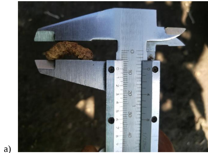
Figure 1. Turmeric rhizome a) width measurement b) Bulk density measurement
