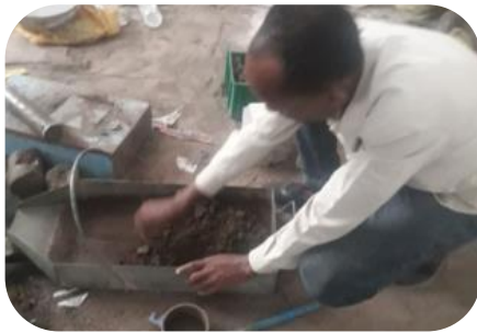
figure(a).mixing soil sample with water for compaction
