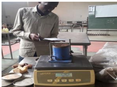
figure(c).determine the weight of compacted soil
