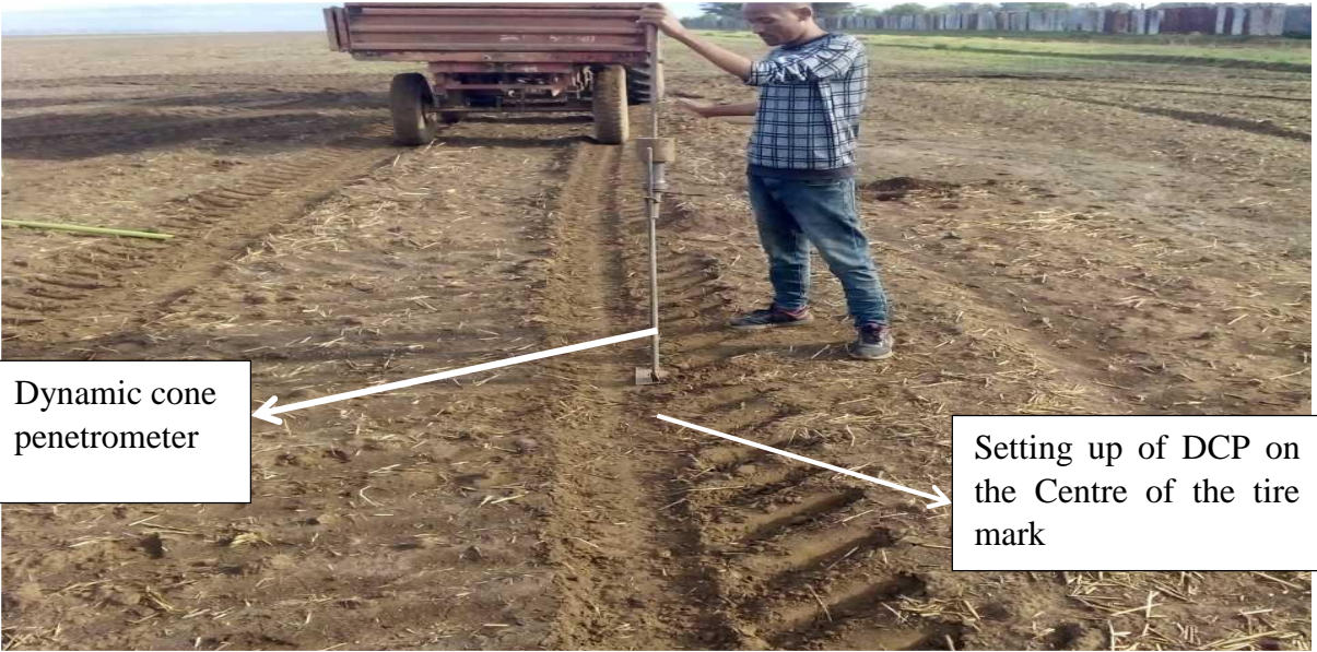
Figure 14. Tire mark's center is measured using a dynamic cone penetrometer.
