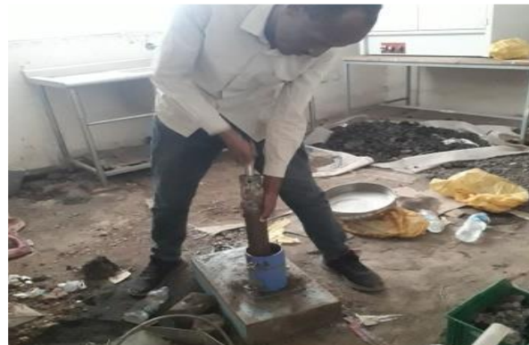
figure(b).compacting the soil
