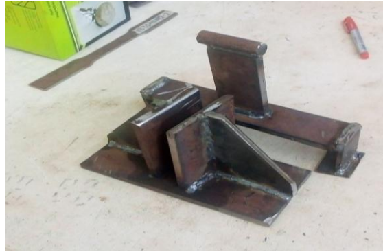
Figure 3.24 3-point flexural bending fixture after preparation
