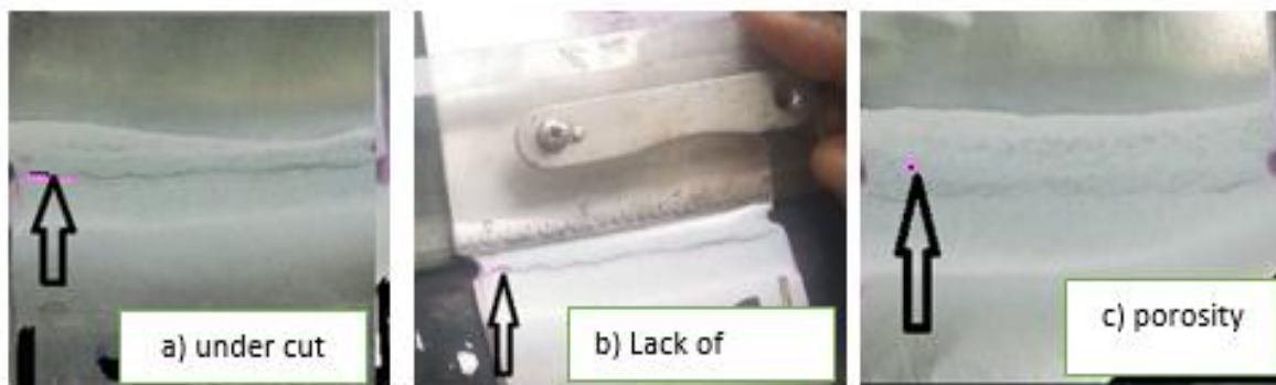
Figure 3.14 defects on dissimilar weld metal: a) sample no.1, b) sample no.2, and c) sample no.13
