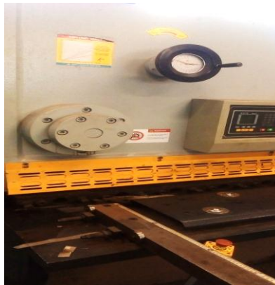
Figure 3.6 shear cutting machine (@ CEE)
