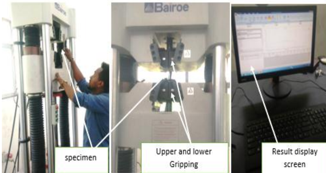
Figure 3.17 tensile test experimental set-up ( at Ethiopian Technical Institute)
