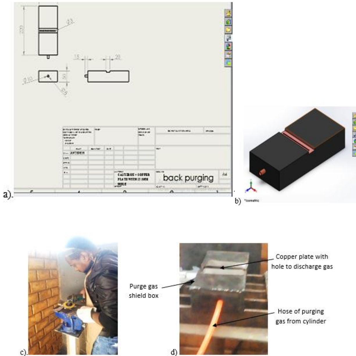
Figure 3.7 Back purging tool a) 2D with dimension b) 3D model c) on device preparation d) finished device
