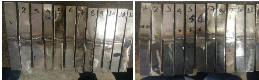
Figure 3.26 some of specimen after sectioned for flexural strength testing
