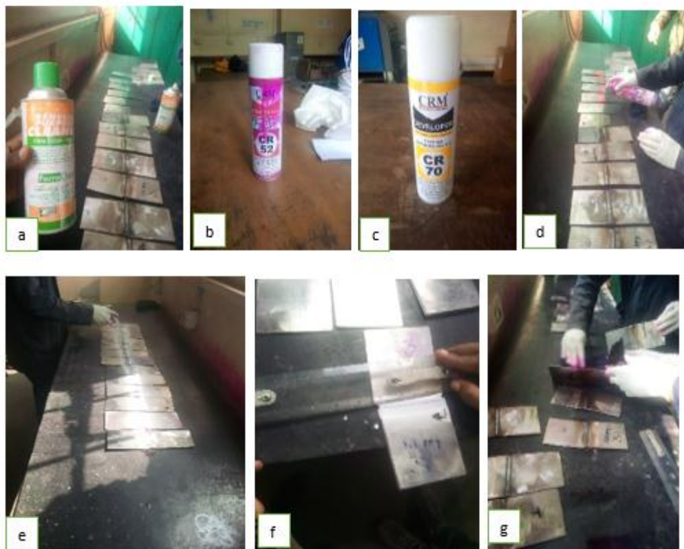
Figure 3.12 PT Processes: a) pre-cleaning samples by using general-purpose cleaner, b) penetrant for segregation c) developer d) Application of a penetrant liquid, e) Application of developer f) Inspection of the test surface, g) post-inspection cleaning (anti-corrosion solutions)
