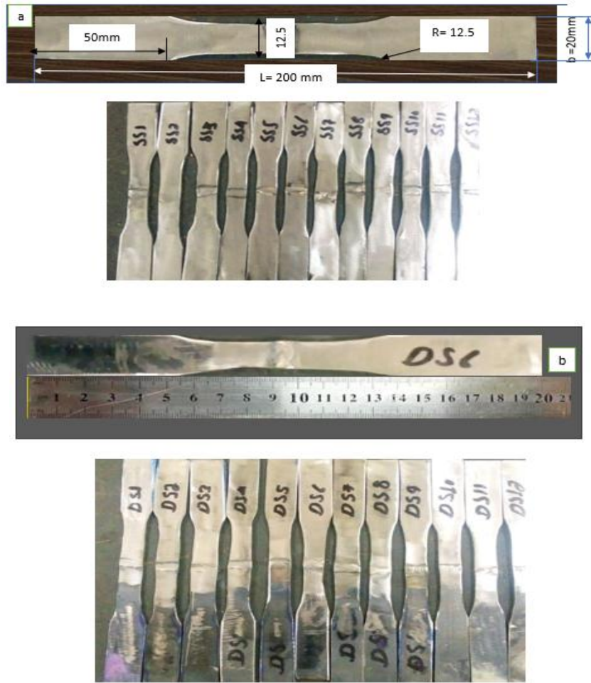
Figure 3.16 sample of specimen prepared for tensile strength: a) for similar, b) for dissimilar
