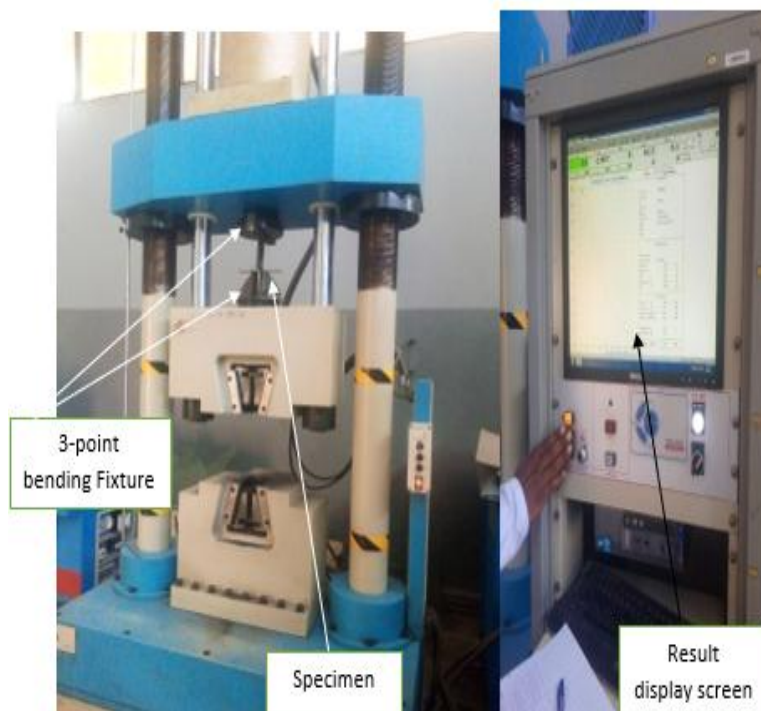
Figure 3.27 flexural testing set up (@ Ethiopian Conformity Assessment Enterprise)
