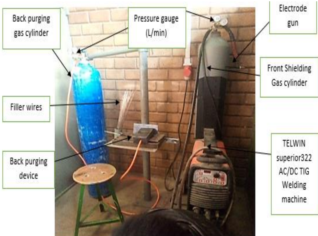
Figure 3.8 Equipment used for TIG welding setup (@ CEE)
