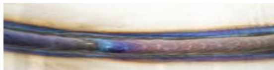
Figure 2.3 back purged weld (Soul performance Products, 2019).
