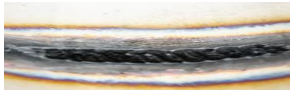
Figure 2.2 oxidation ( sugaring) (Soul performance Products, 2019).
