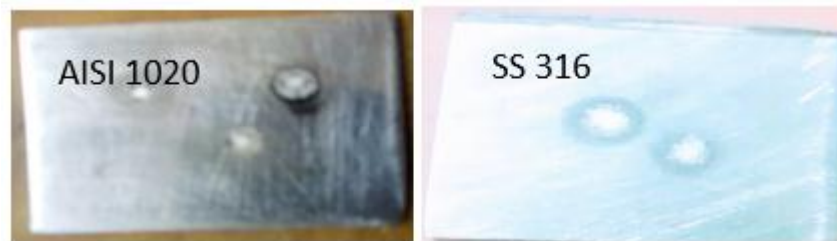
Figure 3.3 specimen for chemical composition after testing
