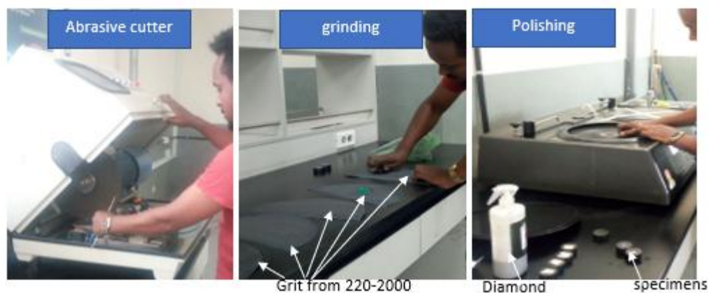
Figure 3.29 preparing a specimen for metallographic analysis
