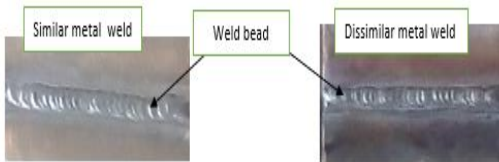
Figure 3.11 weld bead of similar and dissimilar welded samples
