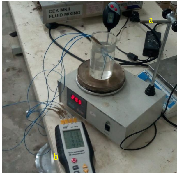
Figure A. 1 Thermometer calibration (a) Reference thermometer (b) K-type 4-channel thermocouple thermometer
