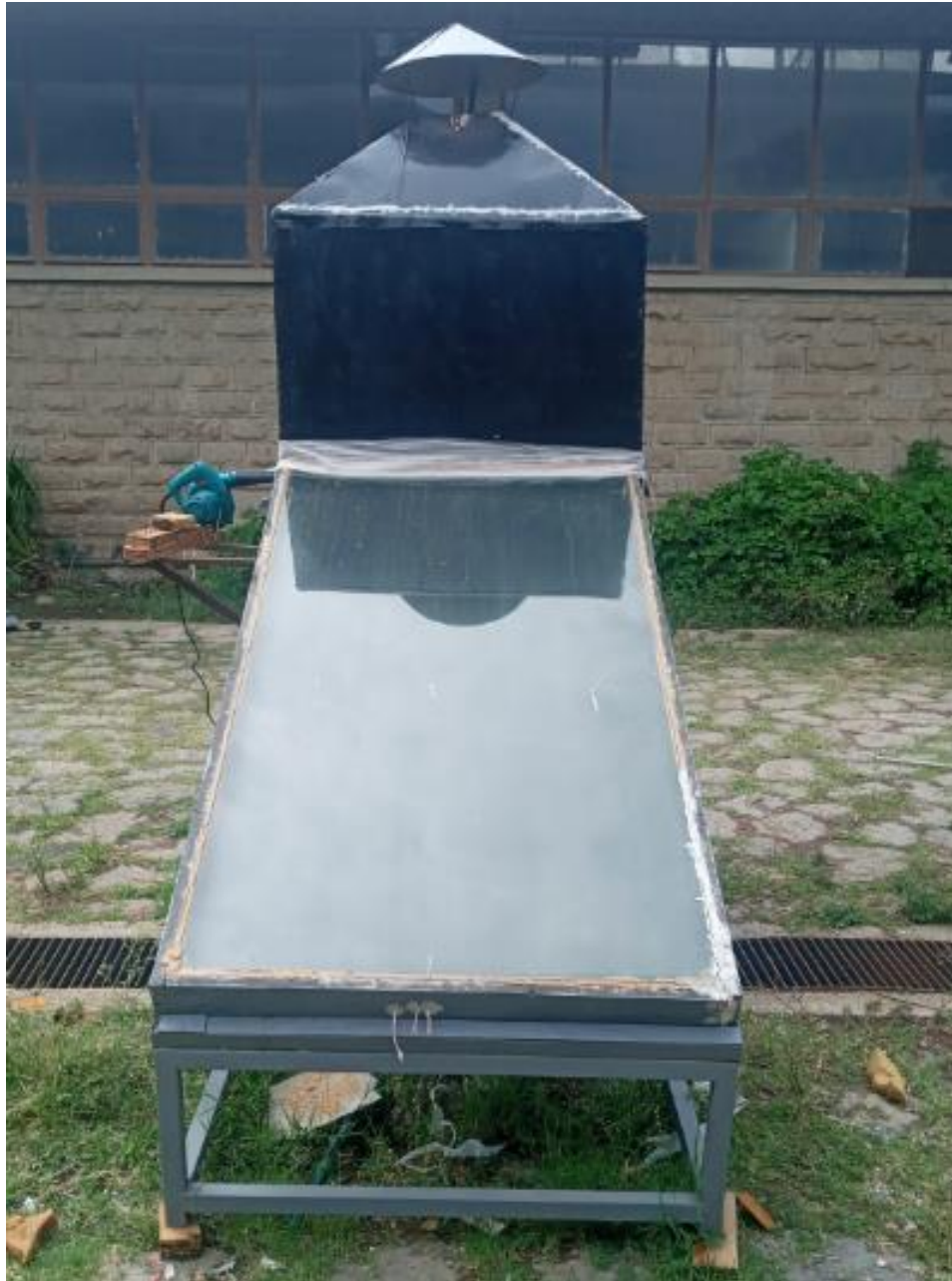
Figure 5.8 Experimental setup of the dryer
