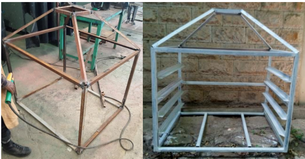
Figure 5.5 Manufacturing process of drying chamber
