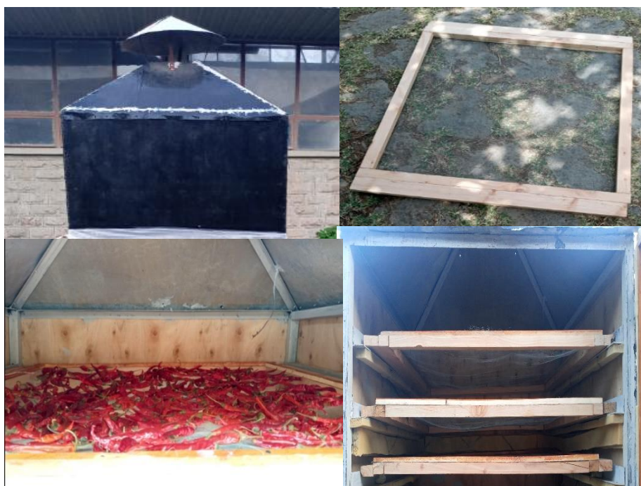
Figure 5.6 Pictorial view of drying chamber and loaded tray
