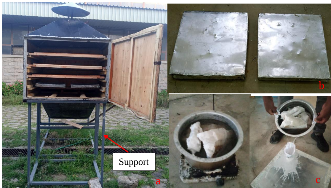
Figure 5.7 (a) Placement of PCM container inside drying chamber, (b) PCM container, (c) filling process
