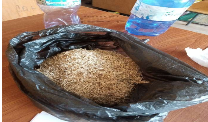
Figure 3.4: cactus fiber after being chopped
