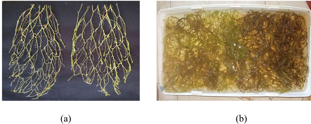
Figure 3.3: cactus fiber preparation (a) cactus fiber pulled out from the cladode, (b) cactus fiber immersed in 0.1N of NaOH
