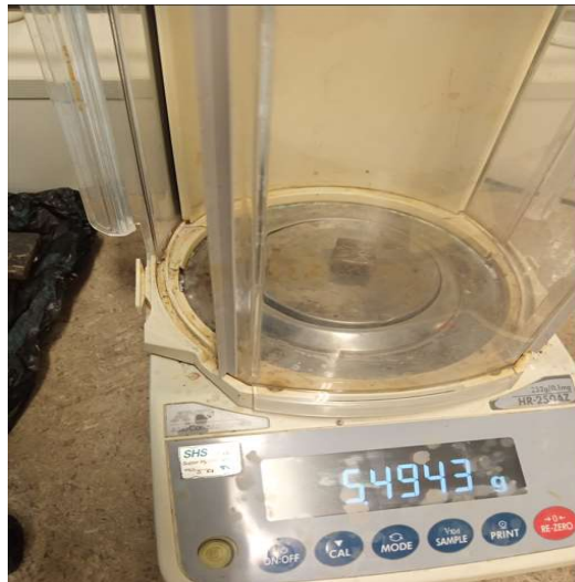
Figure 3.19: Digital balance used to measure specimens for moisture absorption
