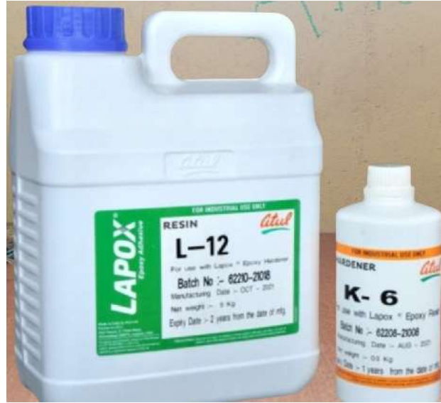
Figure 3.8: Epoxy resin and hardener for sample preparation
