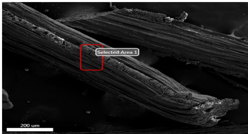
Figure 3.5: SEM image of cactus fiber
