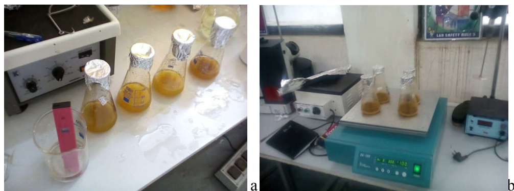
Figure 6 a) PH Adjustment using Hanna PH 210 Micro Processor PH Meter b) mixture of adsorbent and adsorbate in a shaker model no SK 300
