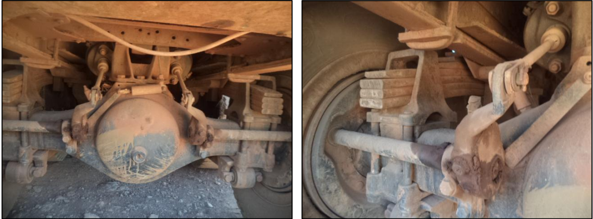
Figure 2.5 Existing manual slack adjuster mounted on the brake system of Sino truck
