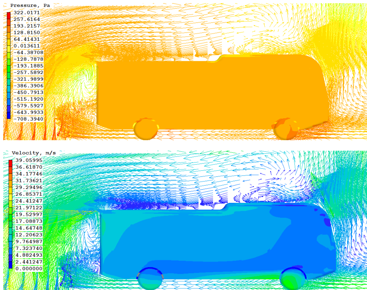
Figure4.9: model 3 velocity and pressure distribution when velocity 60km/h
