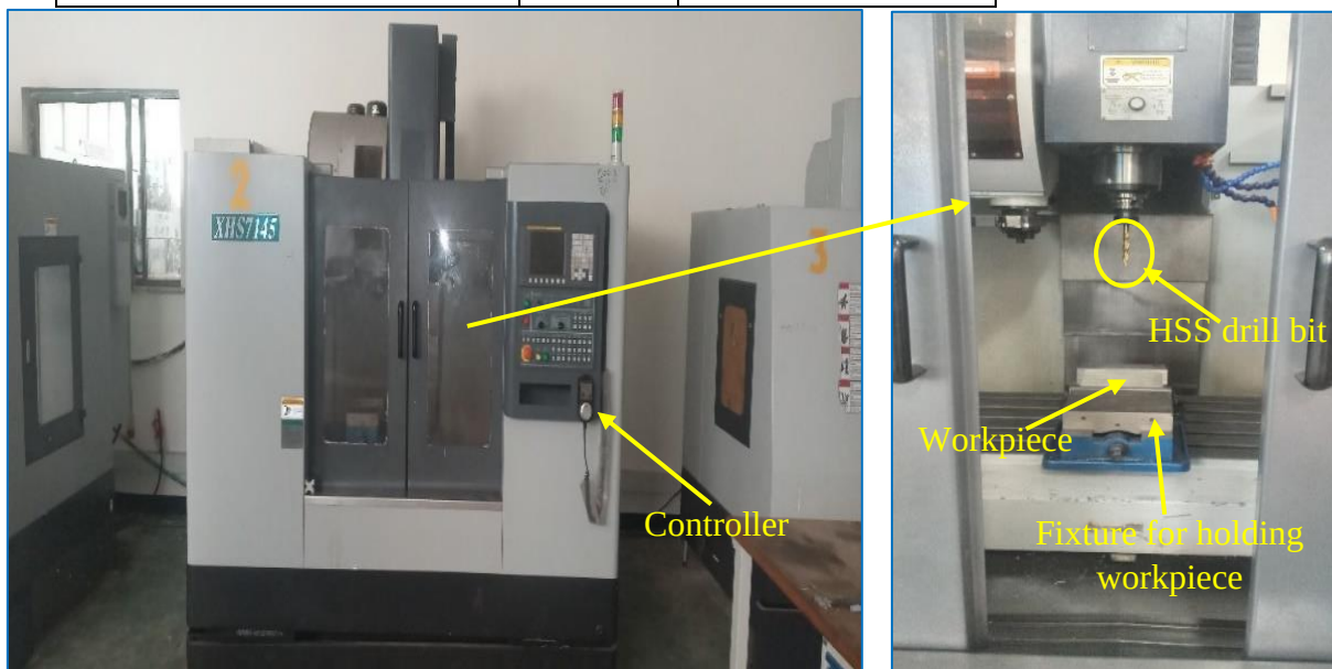
Figure 3.4: Experimental setup of machining the composites (CNC vertical milling)
