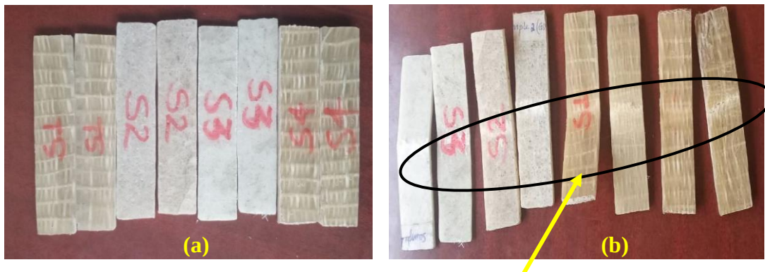
Fracture area of flexural samples
