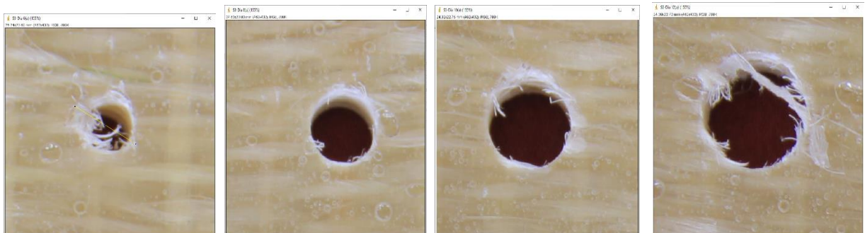
(b) Exit Delamination
