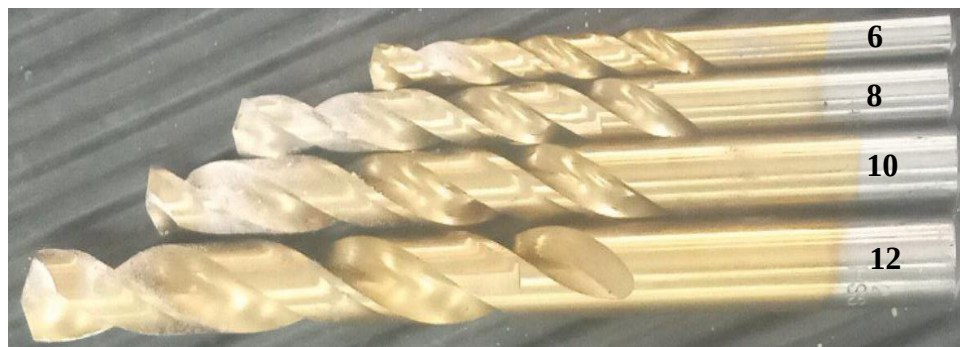
Figure 3.5: Different diameters of the HSS drill bit
