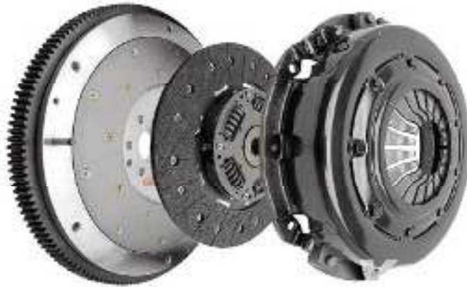
Figure 2.1: Components of the friction clutch
