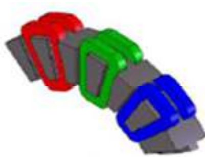
Figure 3.11: Double flux axial stator structure (Peifeng, 2016).
