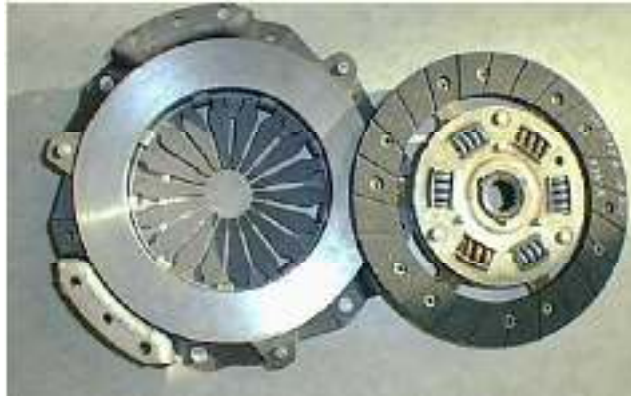
Figure 4.1: Toyota 3L, manual transmission clutch system.
