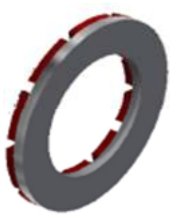
Figure 3.21: 3D view of the armature plate
