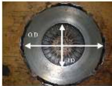
Figure 3.2: Toyota 3L, clutch main dimension
