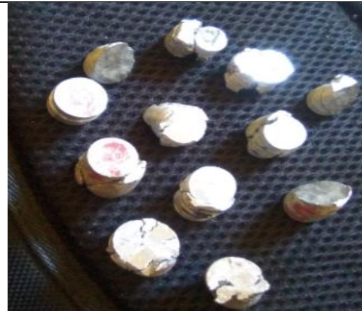
Figure 5. 7 Failure of compression test samples
