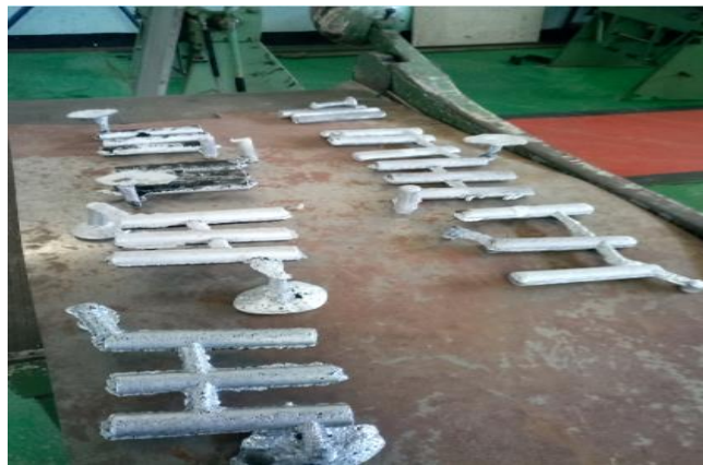
Figure 5. 1 Manufacturing of Al/SiC-bagasse ash composite
