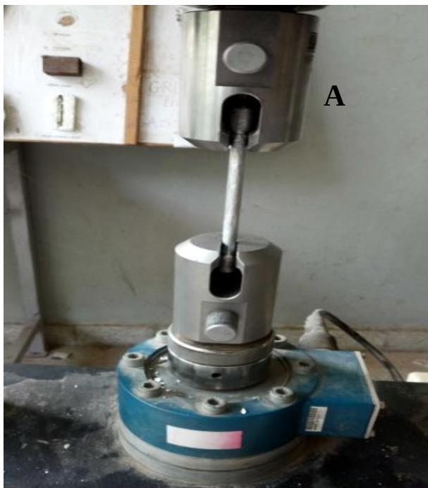
Figure 5. 3 (A) Tensile test set up on UTM
