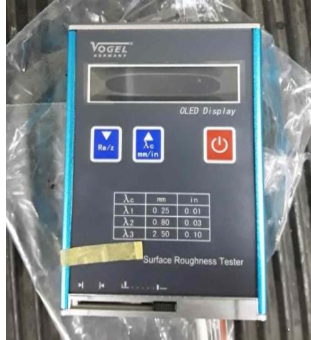
Fig. 3.5. Photograph Image of contact type Surface Roughness Tester with Model 657111
