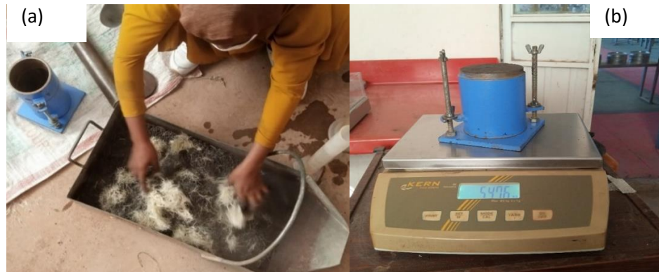
Figure 3.4 Photographic view of dry mix of soil, BA, and SF (a), Compacted mix(b)
