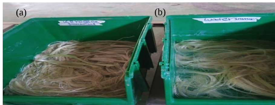
Figure 3.7 Photographic view of kerosene immersed (a) and water immersed sisal fiber (b)
