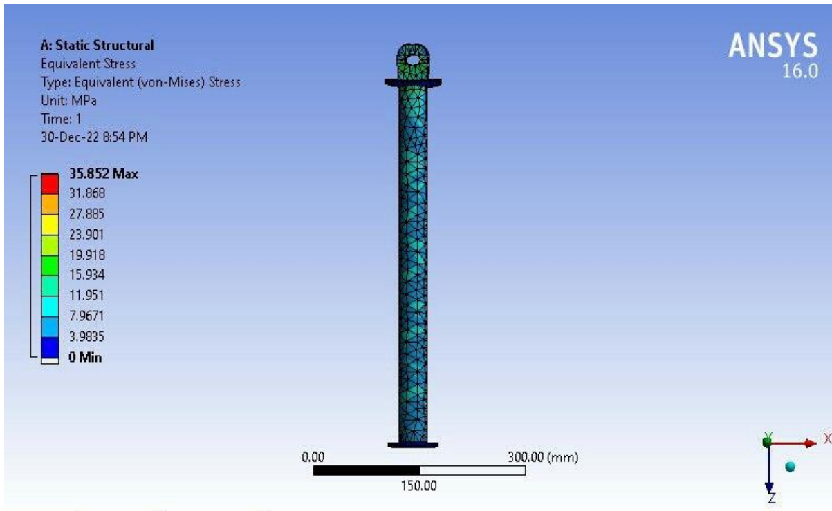
Figure III. 5. Analysis result of the piston rod model with a mass 10kN
