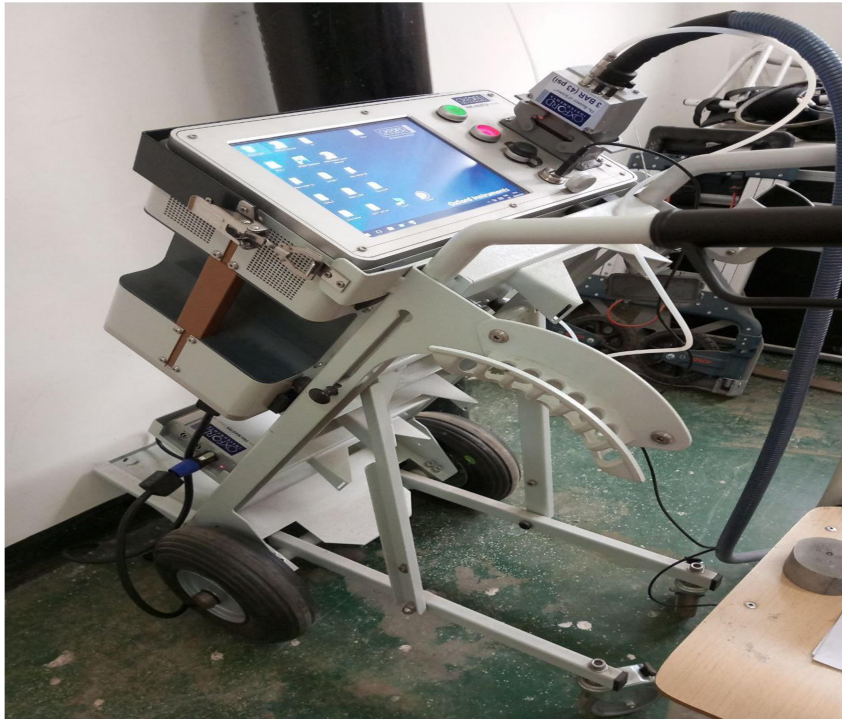
Figure 3-2 Spectrometry used to identify Chemical Composition
