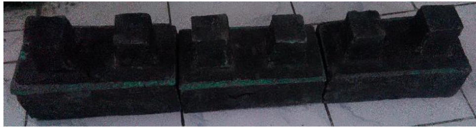
(a) Interlocking Bricks
