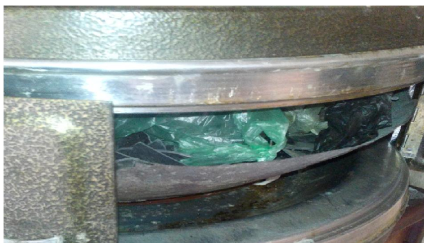
Figure 3.37 putting the waste plastic in heater
