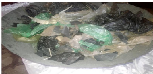
Figure 3.36: Loading of waste plastic on the Aluminum plate
