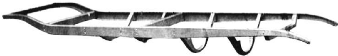
Figure 2.1 grillage chassis of a car at the beginning of 20 century, made of stamped steel
