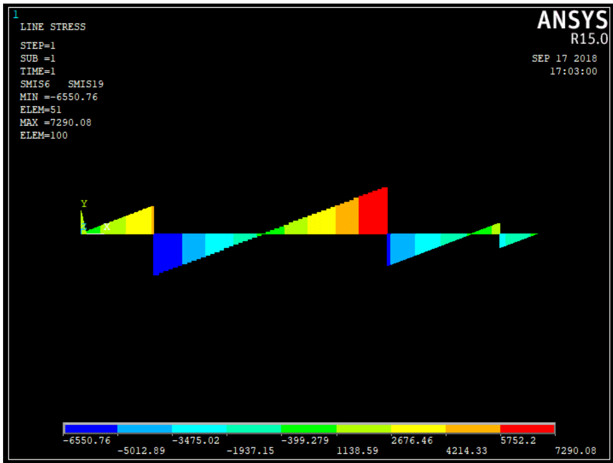
Figure 4.12. Shear force Result diagram using ANSYS
