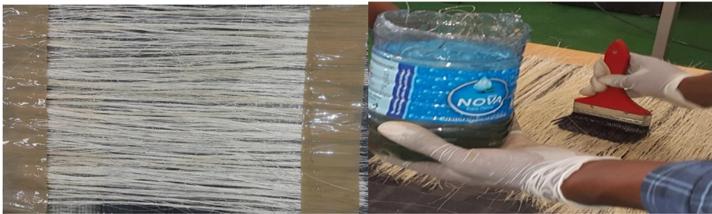
Figure 3-10 Preparation of Laminate by hand layup method
