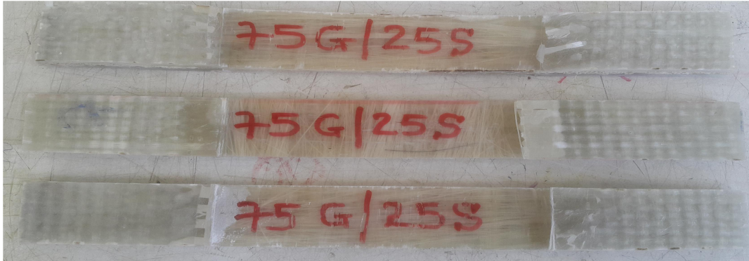
Figure 4-6 75 % Glass Fiber and 25% Sisal Fiber Specimen for Tensile Test
