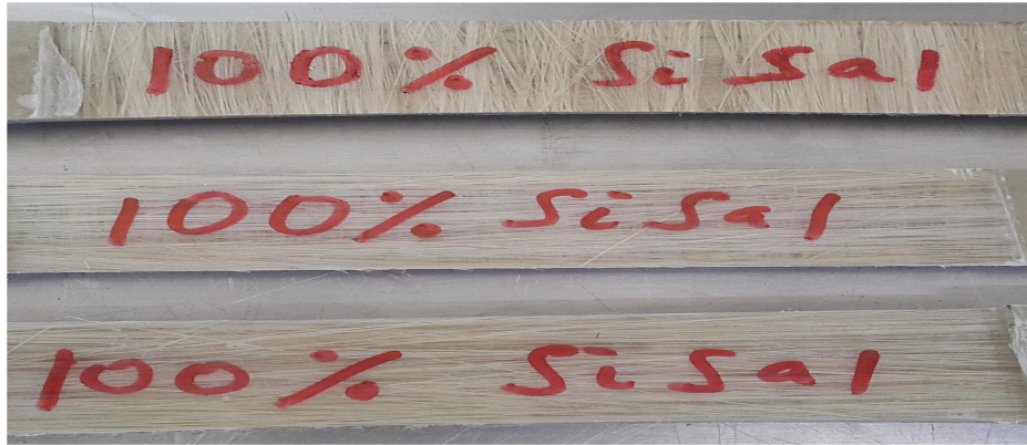
Figure 4-18 100% Sisal Fiber Specimen for Flexural Test
