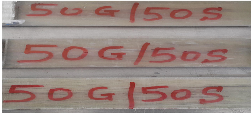
Figure 4-14 50% Glass Fiber and 50% of sisal fiber Specimen for Flexural Test
