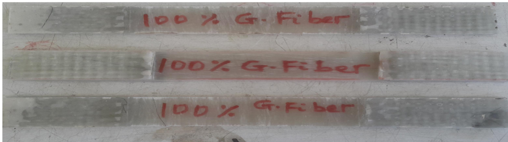
Figure 4-2 100% Glass Fiber Specimen for Tensile Test
