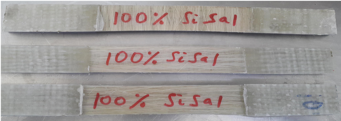
Figure 4-4 100% Sisal Fiber Specimen for Tensile Test
