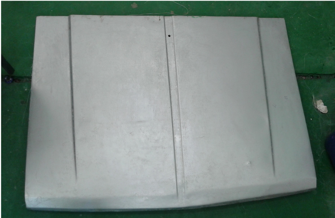
Figure 4-20 Car body panel used for mold preparation
