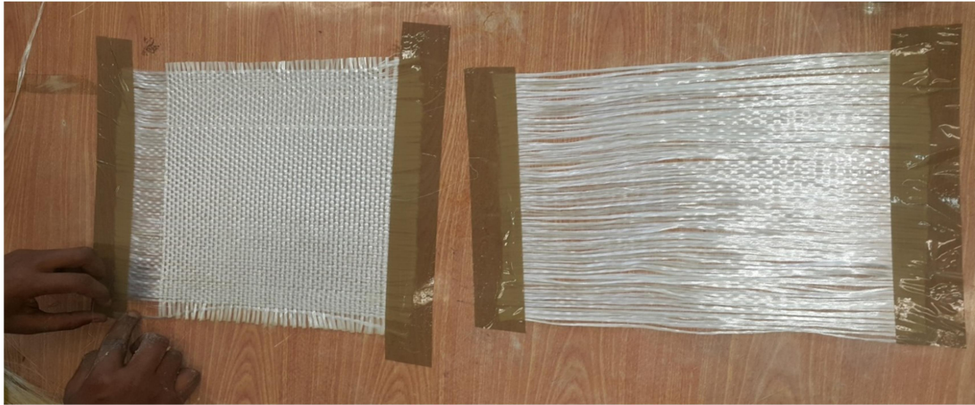
Figure 3-12 Preparation and Cutting Fibers to Desired Dimensions.
