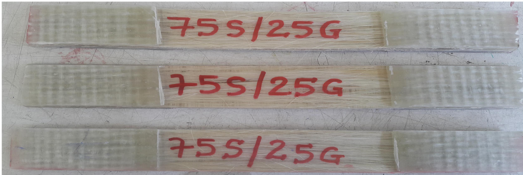
Figure 4-8 75 % Sisal Fiber and 25% Glass fiber Specimen for Tensile Test
