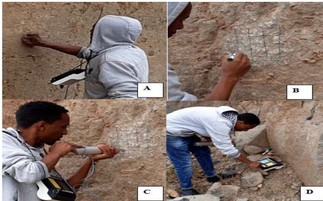
Figure 4.2: Schmidt hammer rebound strength test: A, clean the surface with corundum stone, B, preparing equally spaced square box, C, conduct test and record rebound number, D, convert rebound number to UCS
